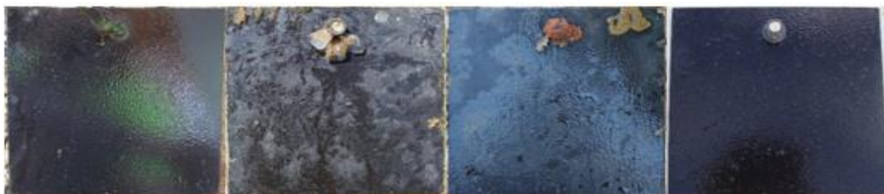
Figure 13: Intersleek® 1100 SR – from Port Orchard, Gig Harbor, Anacortes, and Seattle (left to right).
