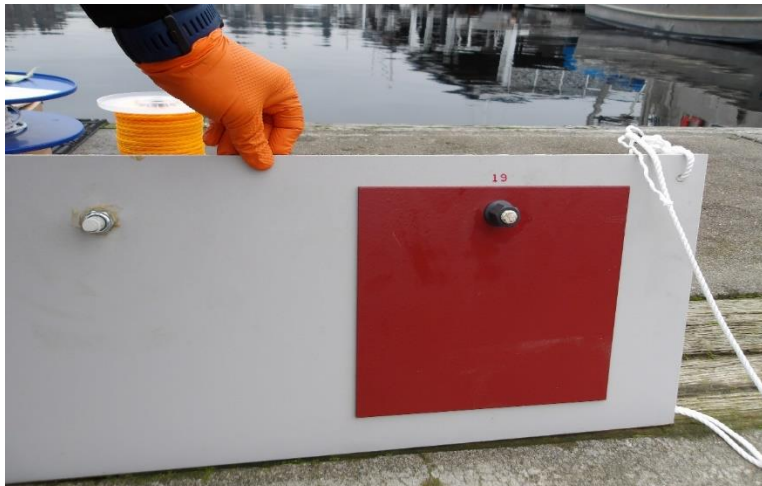
Figure 2: Test panels mounted on the rack prior to submerging into water at Seattle, WA.
