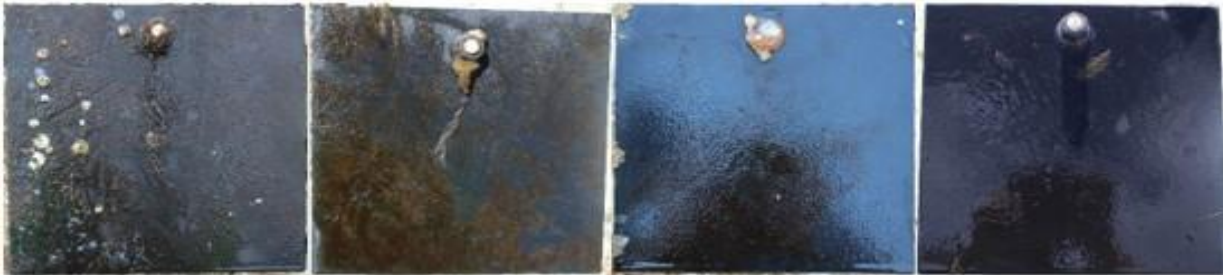
Figure 11: SN-1 – from Port Orchard, Gig Harbor, Anacortes, and Seattle (left to right).
