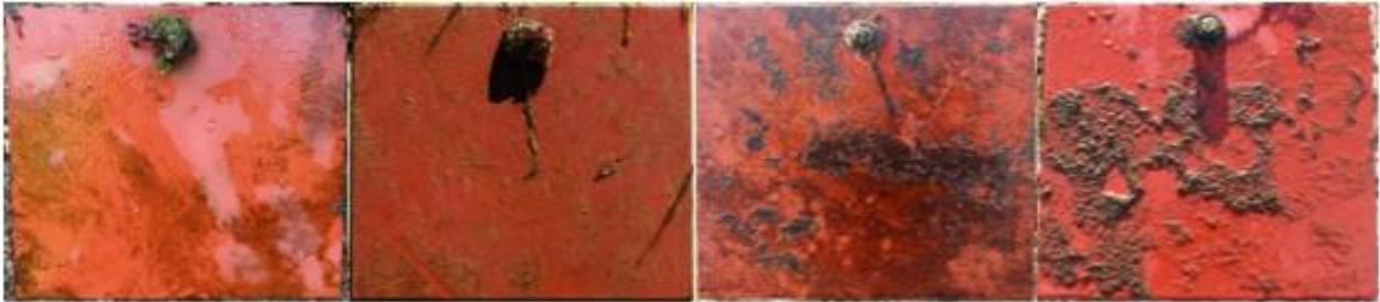
Figure 20: Fiberglass Bottomkote® NT – from Port Orchard, Gig Harbor, Anacortes, and Seattle (left to right).
