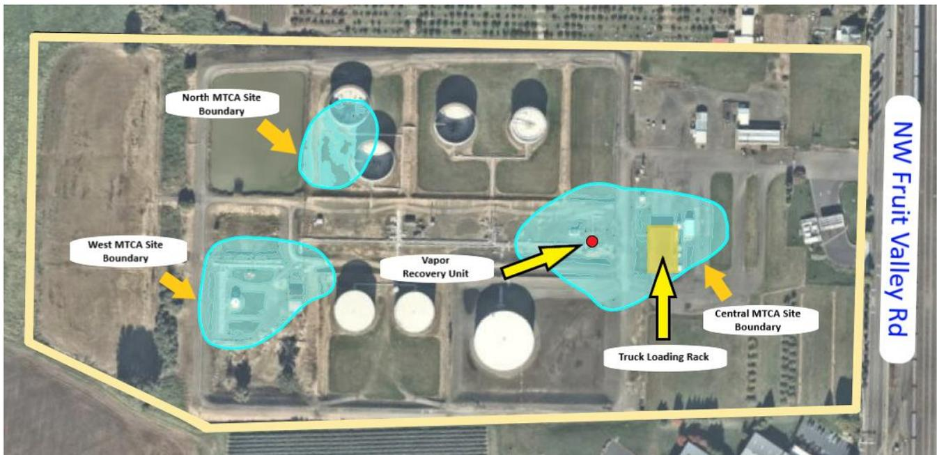
Figure 1. The yellow line marks the boundary of the ST Services NuStar Energy LP property. The blue areas indicate the MTCA Site boundaries. The orange rectangle in the central MTCA Site boundary area indicates the truck loading rack area. The red dot is the location of the Vapor Recovery Unit.
