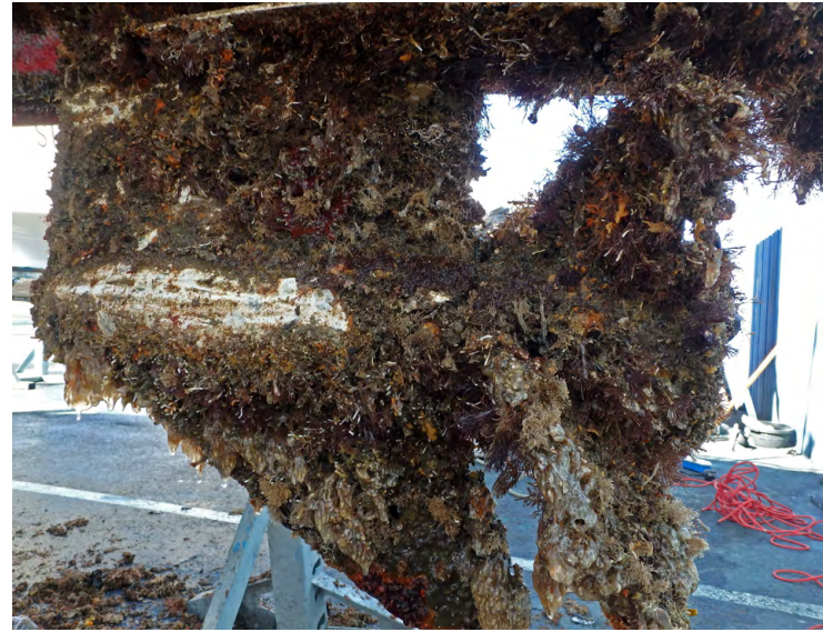
Fouling on propeller
