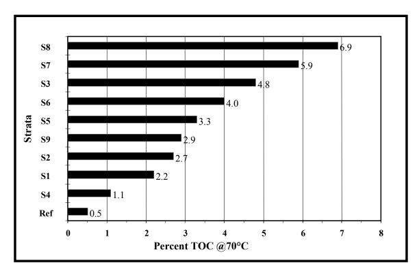
Figure 4. Average TOC Levels in Inner Shelton Harbor Wood Characterization Strata.
