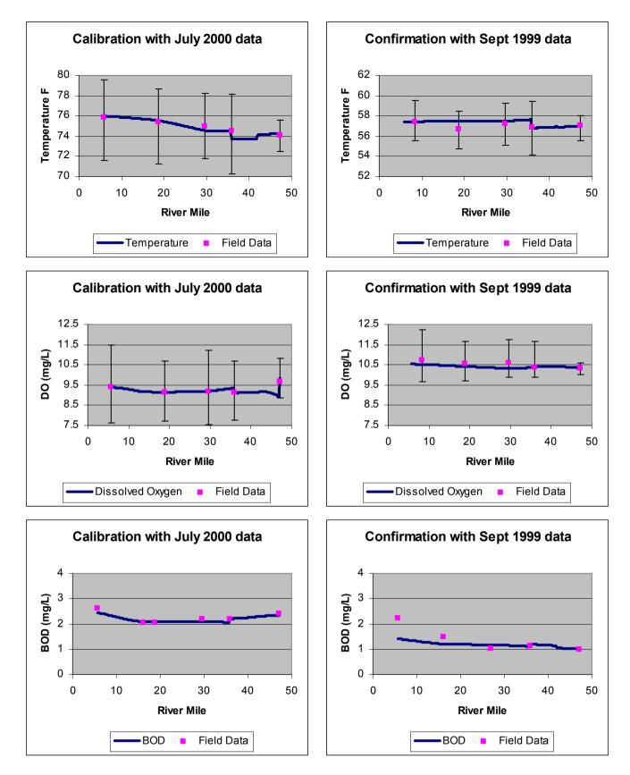
Figure 7. Calibration and confirmation of QUAL2E for prediction of temperature, DO, and BOD in the lower Yakima River during September 1999 and July 2000 (vertical lines are observed means and ranges).
