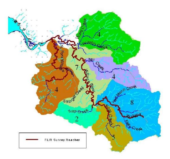
Figure 3. FLIR survey reaches and proposed number of temperature data loggers located in each subbasin
