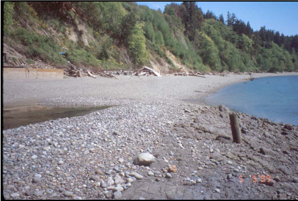
Figure 38. Toe of eastern portion of landslide, showing uplifted beach. Note ponded water in mid intertidal and distorted clays in uplifted portion. [Photo: 5/5/1999, #99-23-16]
