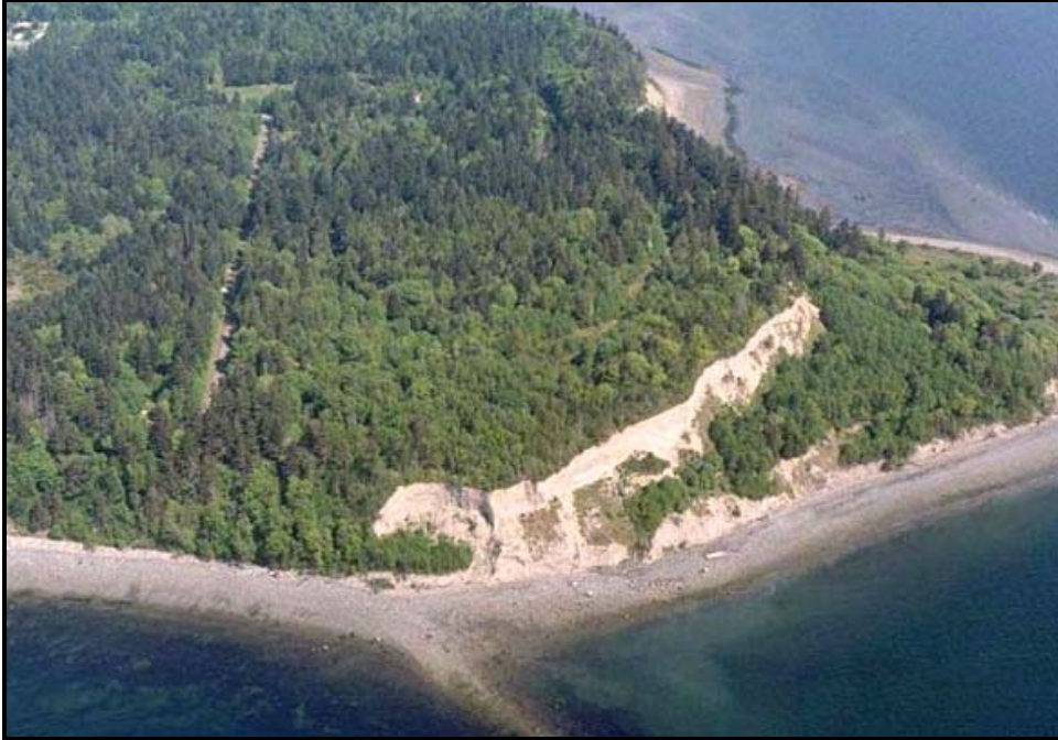
Figure 41. 1994 photograph of large landslide complex at southeastern end of Point Roberts, prior to 1999 failure. Lilly Point is at right edge of photo. [Ecology, 4/28/1994, WHA#022]
