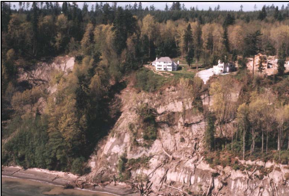
Figure 24. Aerial photo of bluff near north end of map in Figure 25. Note active landsliding, distinct mid-slope bench, distorted stratigraphy, and relatively new homes located along top edge of the bluff. The site described in the text is located at the left margin of the photograph. [Photo: Len Palmer, 4/1997]
