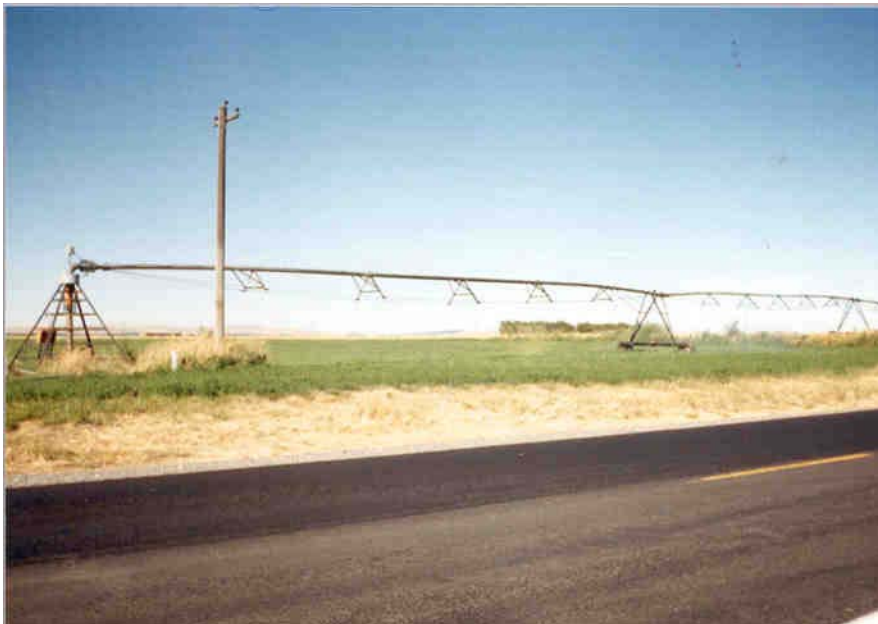
Photo 3: Most irrigation in the Columbia Basin Irrigation Project area is by overhead sprinkler.
