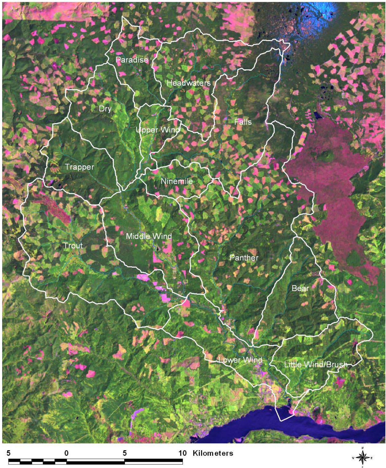
Figure 6. False color Landsat image of the Wind River watershed from July 7, 1991 (TM bands 5,4, and 3).
