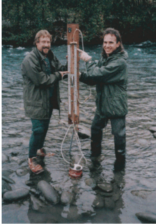
Figure 8. Demonstration of how a manometer board is used for measuring hydraulic head difference between surface water and ground water head. In this case, the hydraulic head representing the river, on the right side of the board, is higher than the hydraulic head representing ground water, on the left side of the board. This condition indicates a downward gradient at the point where the mini-piezometer penetrates the streambed. Photograph taken by Kirk A. Sinclair, Washington State Department of Ecology, 2002.
