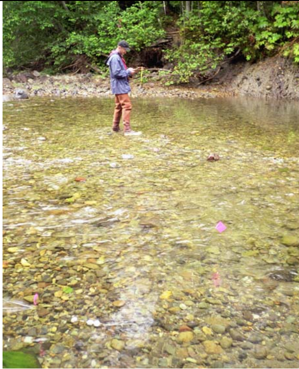
Figure 23A. Greenwater cross-section #1. Taken 10/7/99. View of scour monitors. Pink flags surround a chinook redd providing protection during data collection. Two scour balls were released during redd construction.
