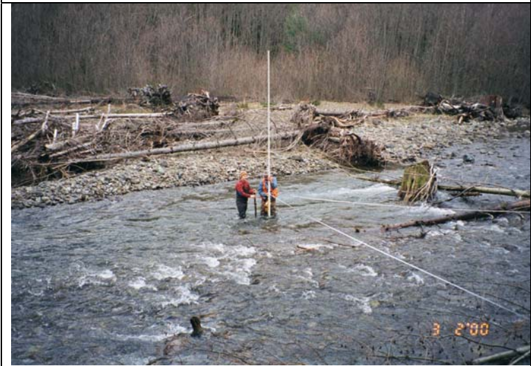
42C. Repeat view of photo 42A for Greenwater redd 1999 #17. Surface scour of 19 cm occurred between the October and March surveys. Photo taken 3/2/00.
