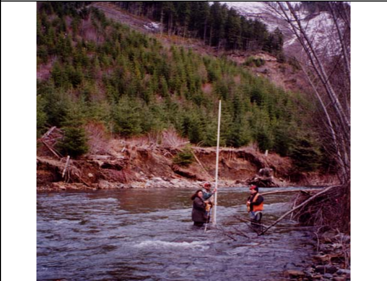
40D. Winter view of Greenwater River chinook redd 1996 #3. Redd is under the survey rod. The late winter survey measured 12 cm of surface scour at the redd site. Photo taken 3/5/97.
