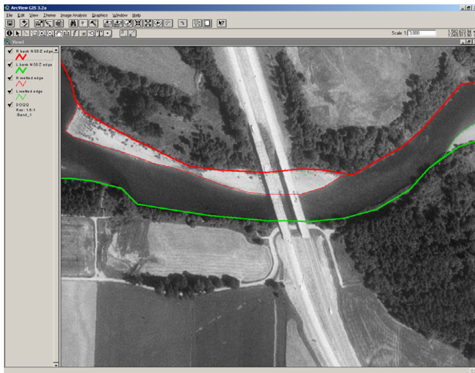
Figure 17. Example of the digital orthophoto quad (DOQ) for the mainstem of the Stillaguamish River at the I-5 bridge and digitized wetted edges and bankfull edges.
