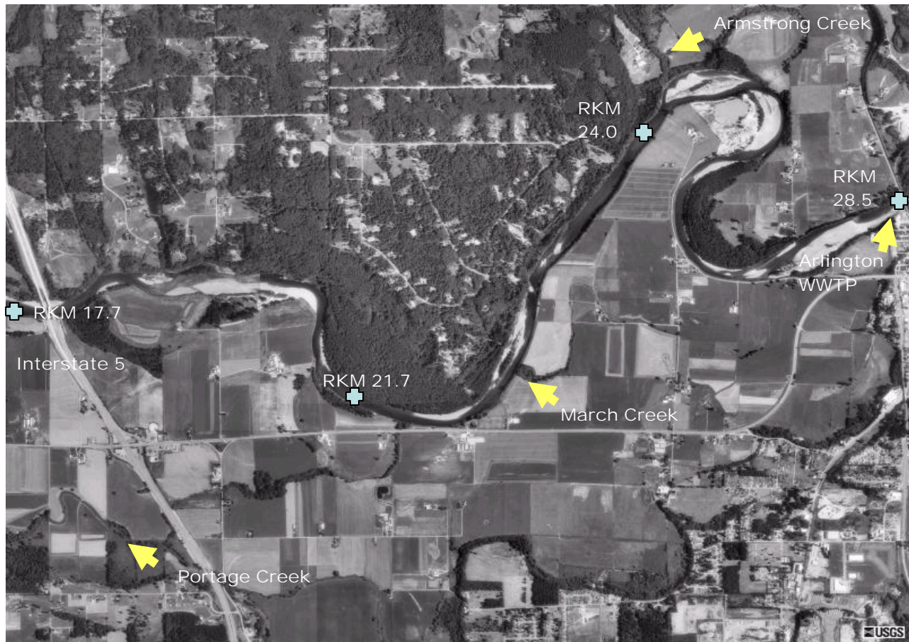
Figure 7. Locations of four diel monitoring probes (broad crosses) in the Stillaguamish River from Arlington to Interstate 5 in September 2000 and October 2001. RKM = river kilometer
