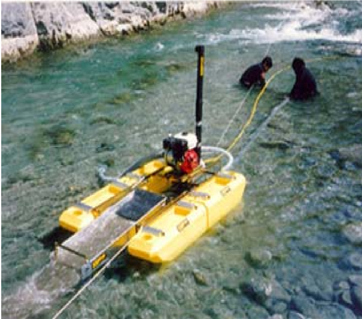
Figure 2. A Typical Gold Dredge
