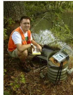
Downloading data from a stream gage
