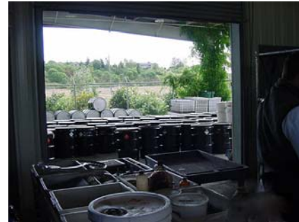
Properly closed drums, stacked with aisle space and under cover are far less likely to cause harmful spills
