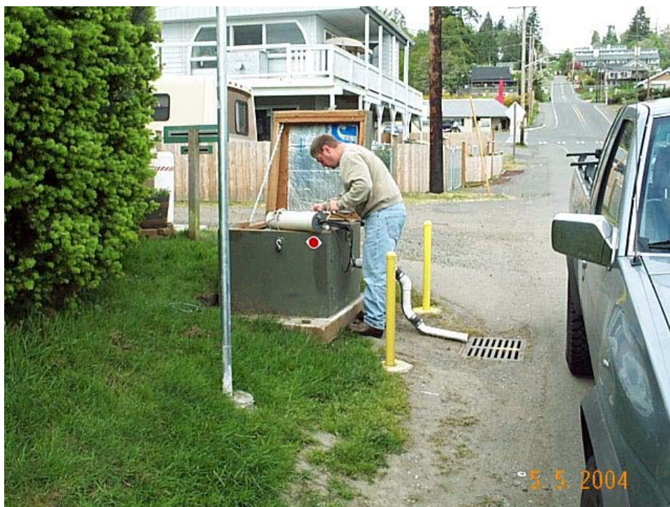
Figure 4-6. Manchester Stormwater Outfall Water Quality Sample Station, Showing Automated Sampling System Enclosure and Sample Pipe
