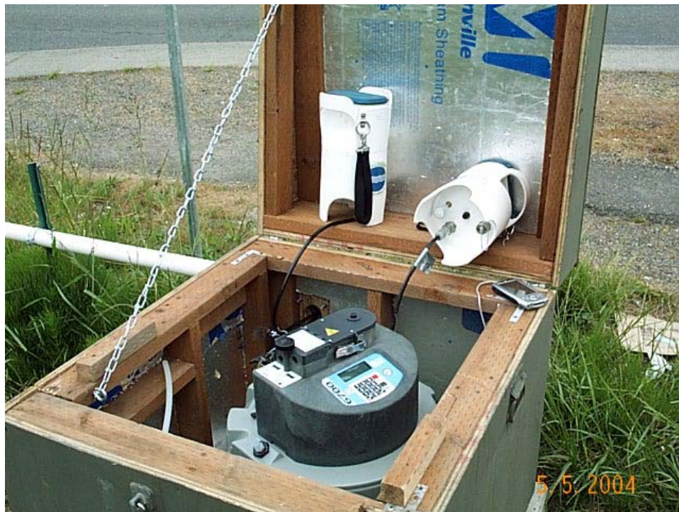
Figure 4-4. Typical Automated Sampling System and Enclosure
