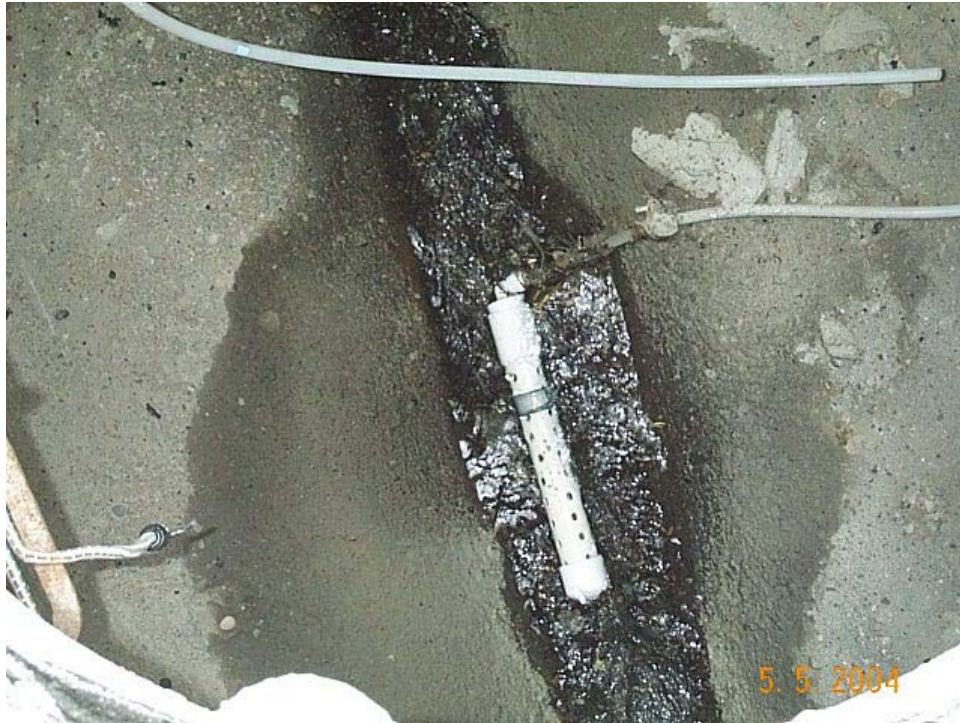
Figure 4-12. Manhole-Type Stormwater Water-Quality Sample Station, Showing Flowmeter
