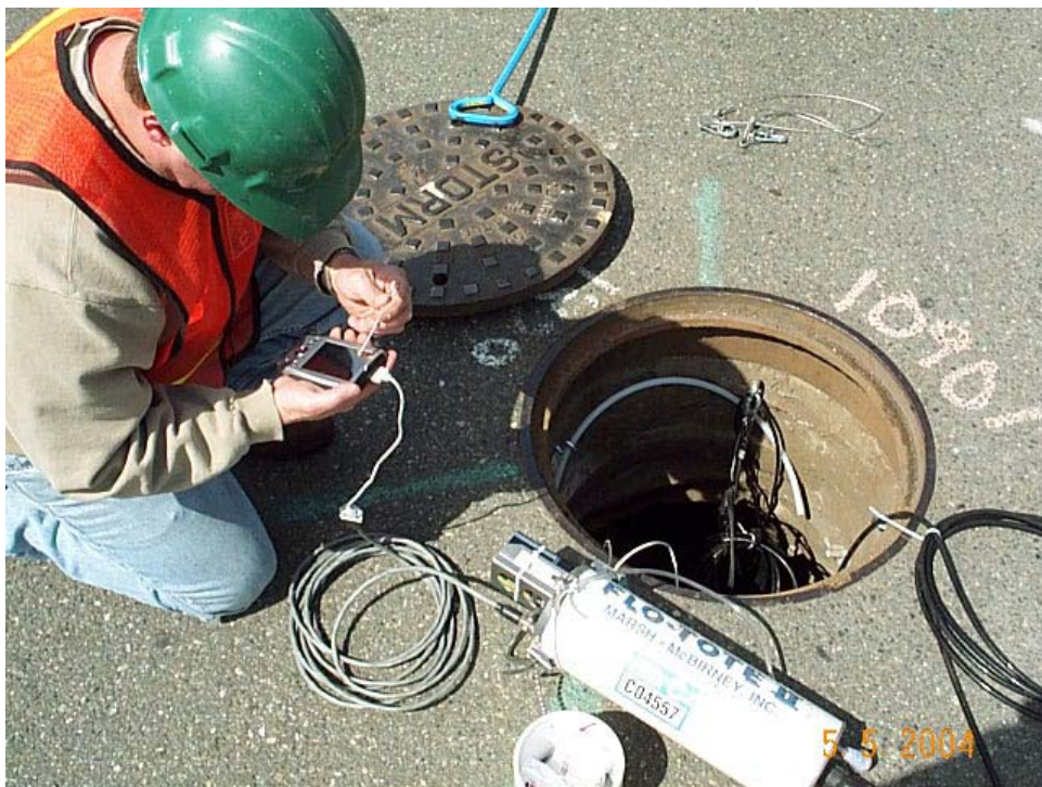
Figure 4-11. Manhole-Type Stormwater Water-Quality Sample Station
