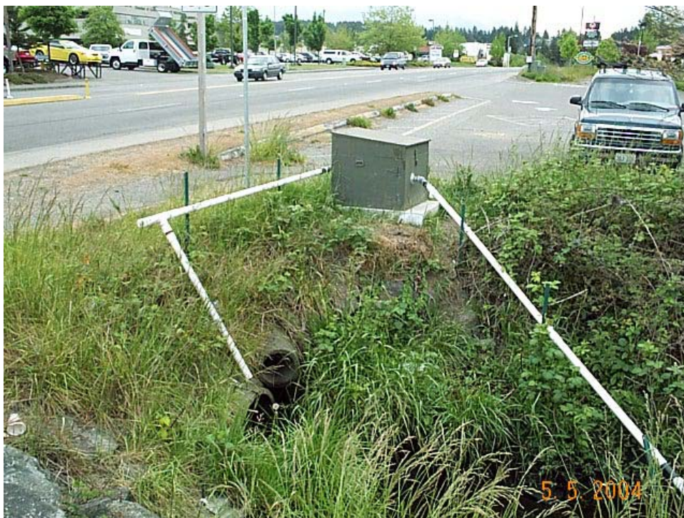
Figure 4-5. Silverdale Stormwater Outfall Water Quality Sample Station, Showing Automated Sampling System Enclosure and Sample Pipe
