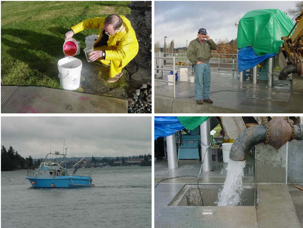
Figure 11. Dye injection study in Port Washington Narrows, clockwise from top left, mixing Rhodamine dye, initiating injection, metering dye into outfall, and tracking plume with vessel.
