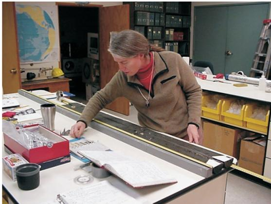
*Fig. 14. Photo of core logging. Sediment properties and sedimentary structures are observed and recorded on core logs.*
