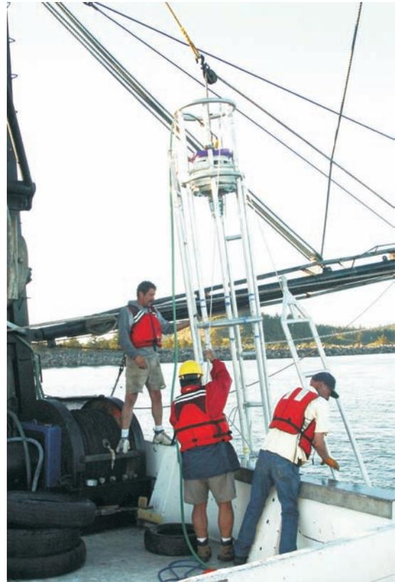
Fig. 5. Photo of crew adjusting the retractable legs of the vibracorer.
