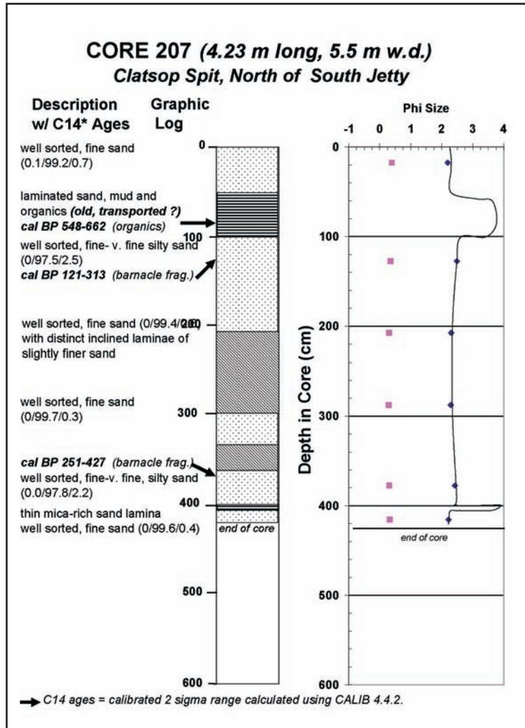
Fig. 29. Descriptive log of core MCR-207.
