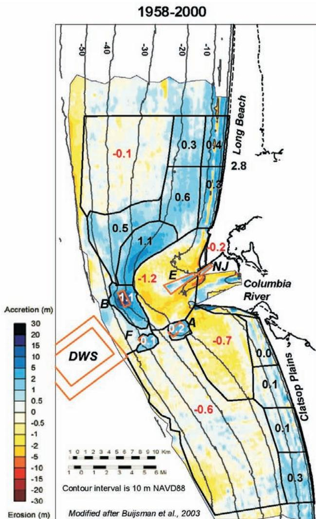
Fig. 46. Bathymetric change during 1958 to 2000 at the MCR. Numbers shown represent volumetric change rates within compartment boundaries in million cubic meters per year.
