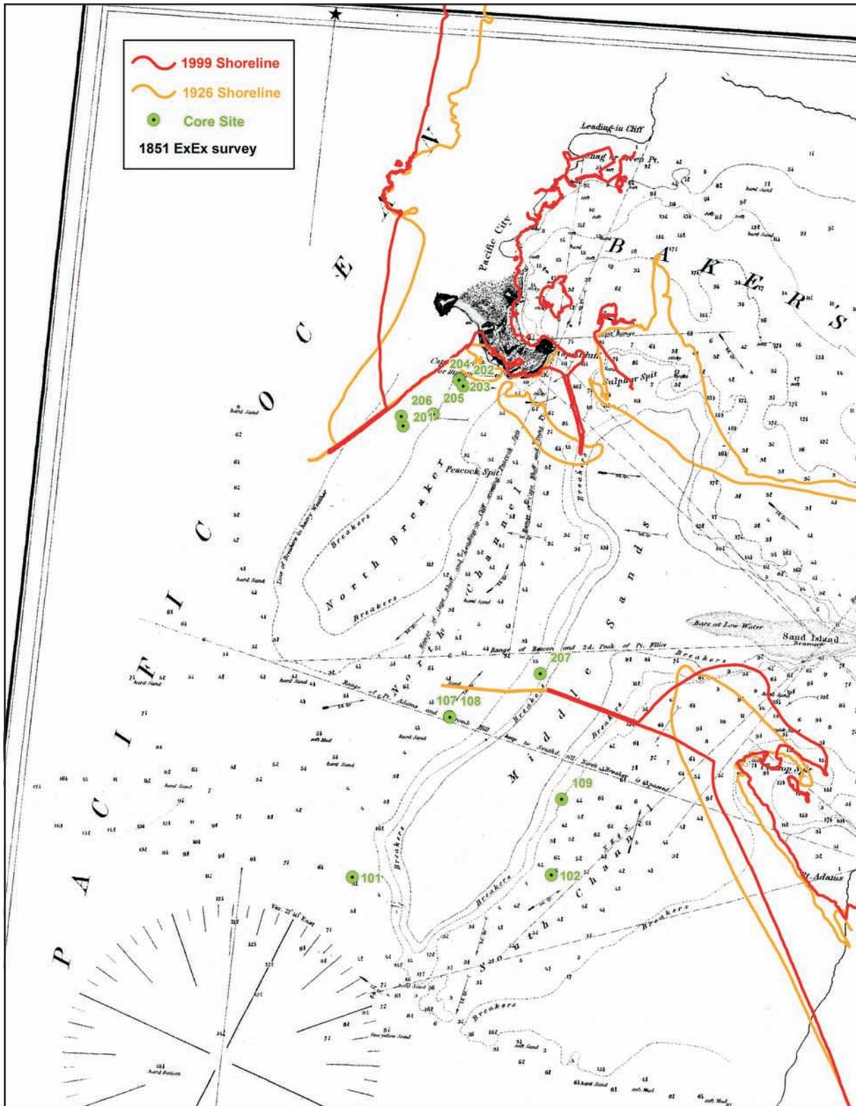
Fig. 18. Vibracore locations, jetties and 1926 and 1999 shorelines plotted on the 1851 U.S. Coast Survey chart, within which the hydrography is from 1850. Depths in channels are in fathoms ( $\geq 3$ ); depths on sand banks are in feet ( $\leq 18$ ) below MLLW.
