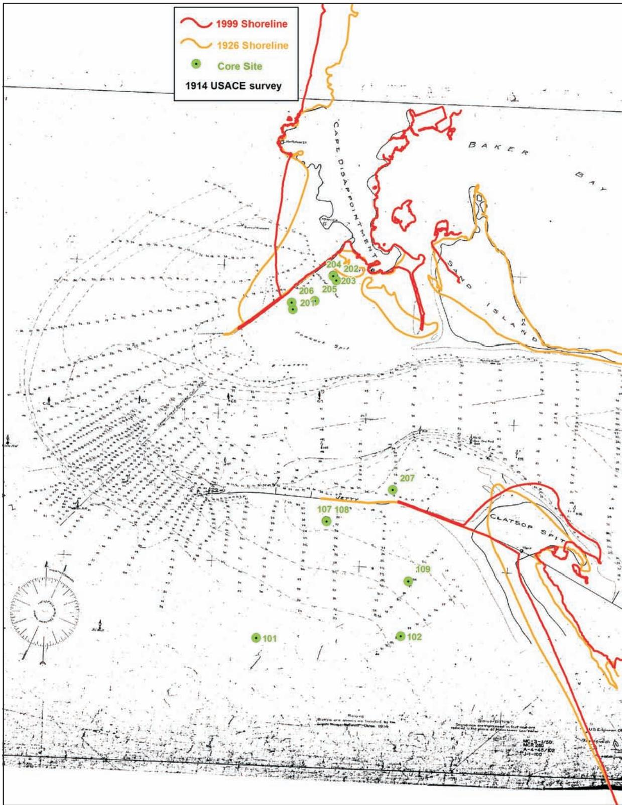
Fig. 22. Vibracore locations, jetties and 1926 and 1999 shorelines plotted on the U.S. Army Corps of Engineers survey MC-1-122 of May 1914. Depths are in feet below MLLW.
