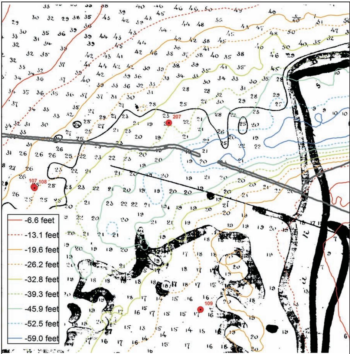
Fig. 43. 1868 bathymetric contours plotted on the 1883 survey along with the 1957 jetty. At the location of the subsequent jetty gap, the channel filled from 59 feet deep in 1868 to 20 feet deep in 1883.
