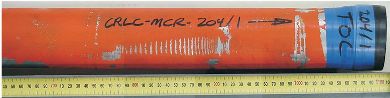
Fig. 7. Photo of scrape marks along a core barrel indicating progressive penetration into the seabed, with the abrasion mark closest to the top of the barrel denoting maximum penetration.
