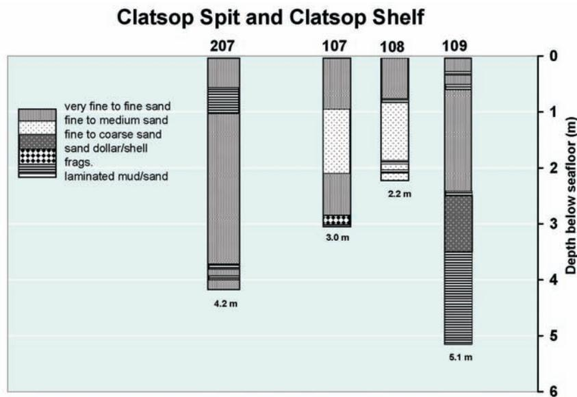
Fig. 36. Core logs showing basic sedimentary units observed in the cores collected along the Columbia River south jetty.
