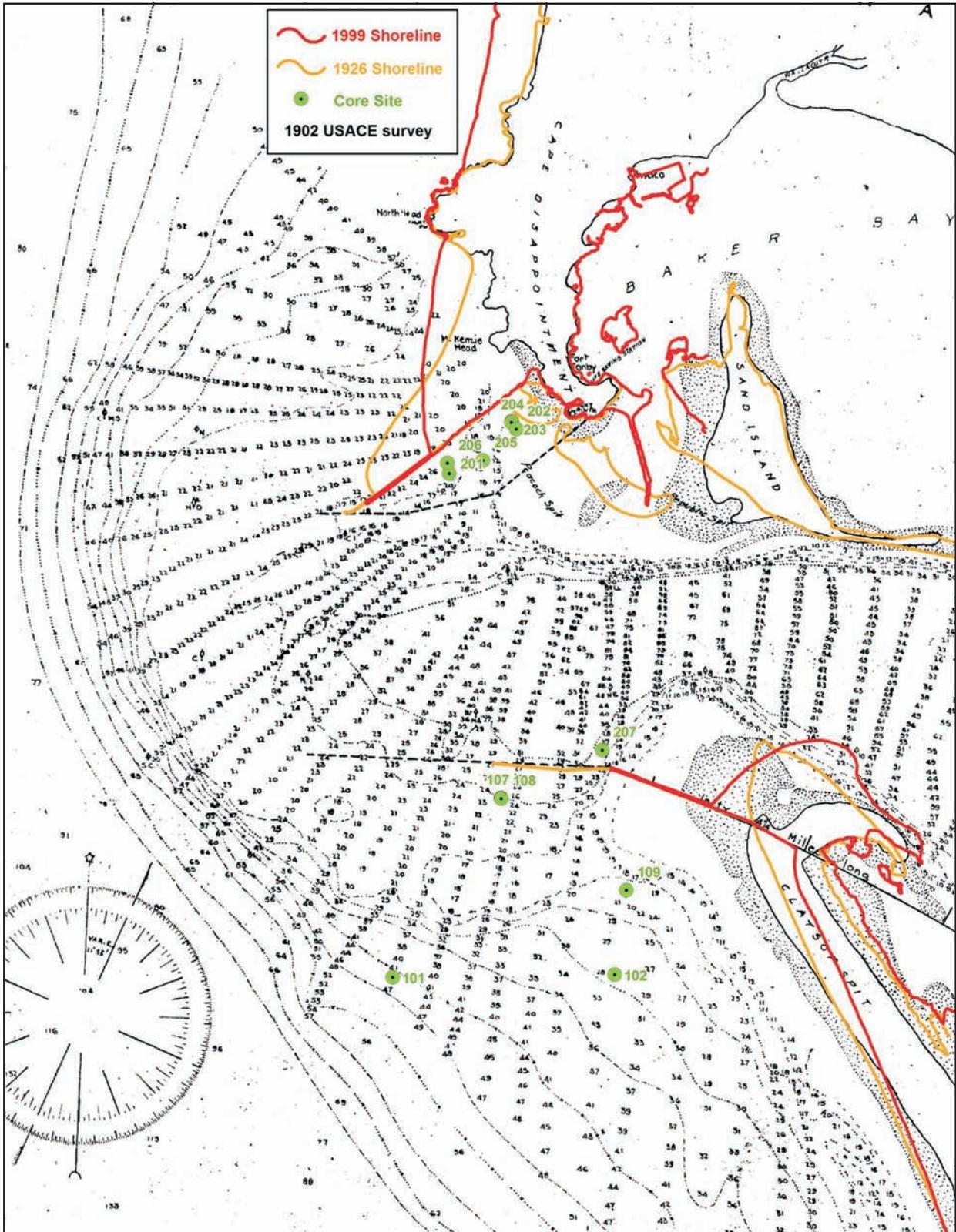
Fig. 21. Vibracore locations, jetties and 1926 and 1999 shorelines plotted on the U.S. Army Corps of Engineers survey MC-1-78 of June 1902. Depths are in feet below MLLW.
