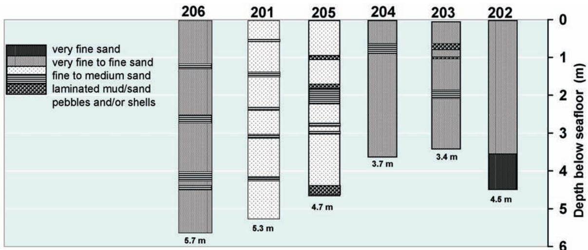
Fig. 37. Core logs showing basic sedimentary units observed in the cores collected along the Columbia River north jetty.
