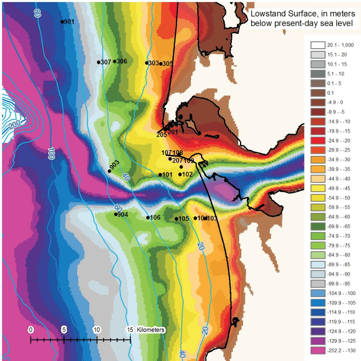
Fig. 38. Vibracore locations, jetties, 1999 shoreline and the modern bathymetric depth contours in 20-m intervals plotted on the lowstand surface (>14,000 BP) interpreted from seismic reflection data (Twichell and Cross, 2001).
