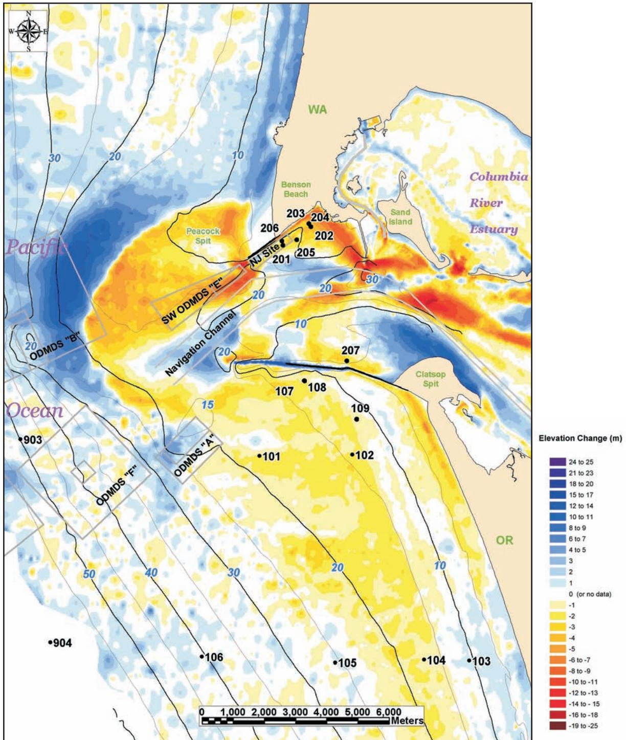
Fig. 24. Locations of vibracores collected in previous study in 2002 by the authors and this project shown with historical bathymetric change from Buijsman et al. (2003) during the period 1926 to 1958 (1935 to 1958 for entrance). Bathymetric contours in meters NAVD88 derived from data from 1998-2003.
