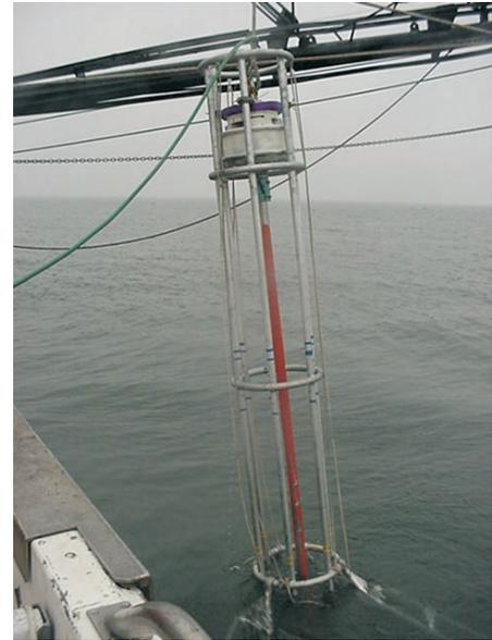
*Fig. 3. Photo of the 7-m high vibracorer (Quaternary Resources, Ltd.) suspended from the starboard outrigger of the "Olympic". The upper 4 m of the tower are shown.*
