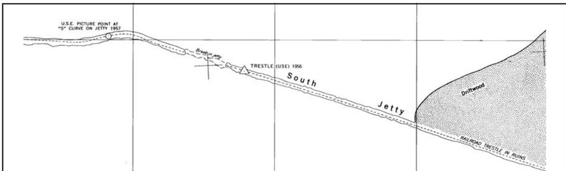
Fig. 44. Deteriorated section of the jetty east of the "knuckle" as mapped on the 1957 National Ocean Service Topographic Sheet (NOS T-Sheet) #10352.
