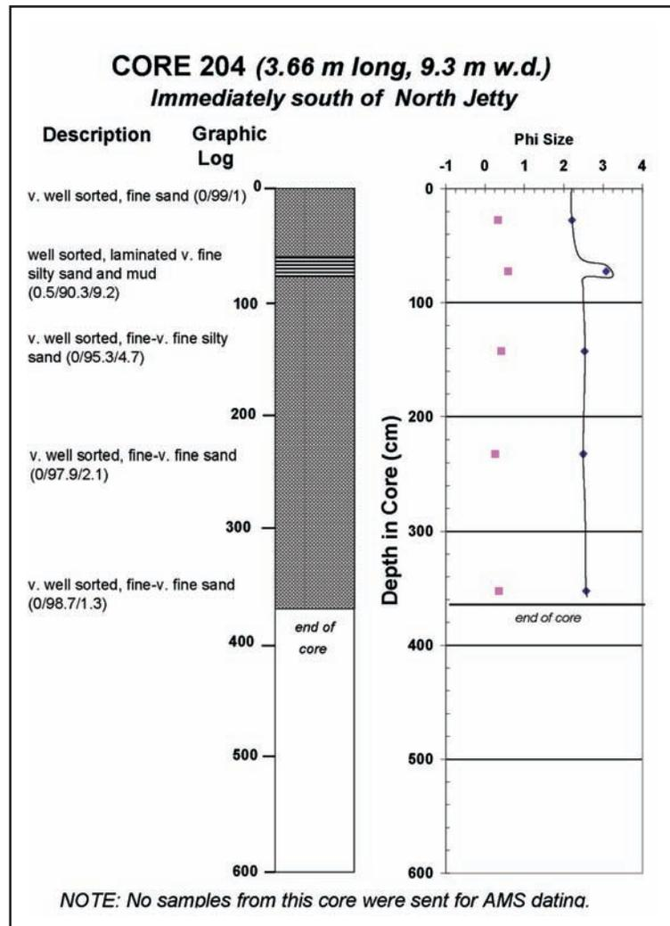
Fig. 33. Descriptive log of core MCR-204.
