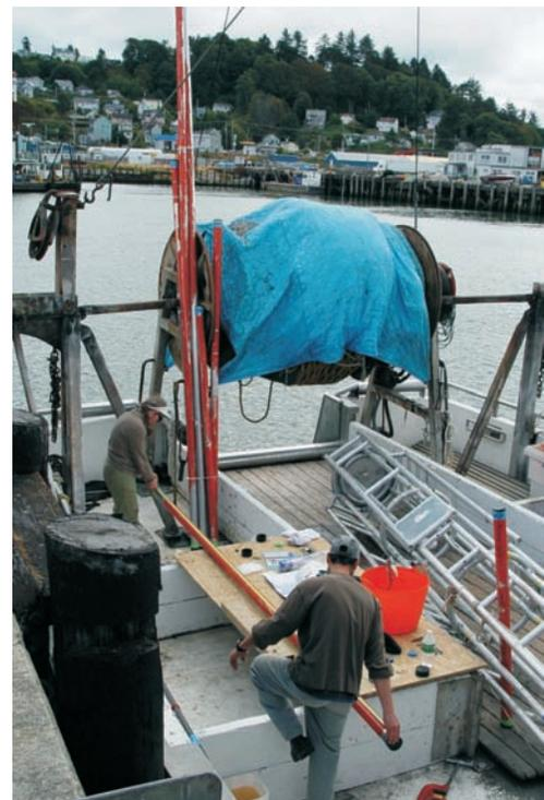
Fig 8. Photo of core processing aboard the "Olympic" while docked at the Port of Astoria. Immediately after collection, cores were secured in an upright position to settle and drain, and within several hours, final measurements of recovery and penetration were made, and each core was then cut into 1.5-m sections for storage in the refrigerated hold of the vessel (photo by R. Gammisch).
