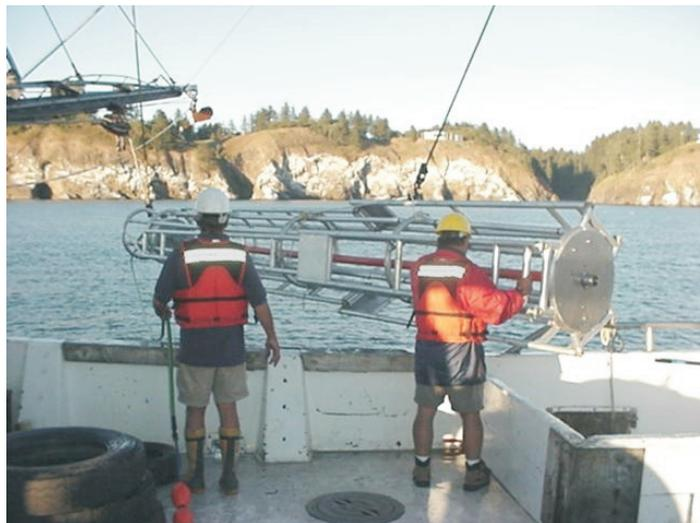
*Fig 4. Photo of the vibracorer suspended above the deck of the "Olympic" for deployment over the starboard side of the vessel.*
