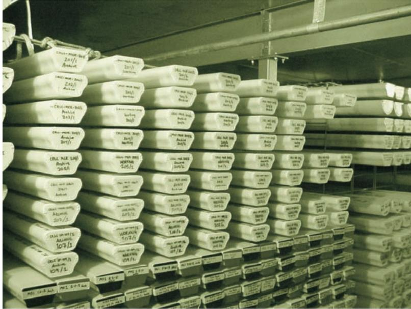
Fig. 16. Photo of the set of archived- and working-half core sections stored in "D-tubes" in the refrigerated facility of the OSU Core Laboratory.
