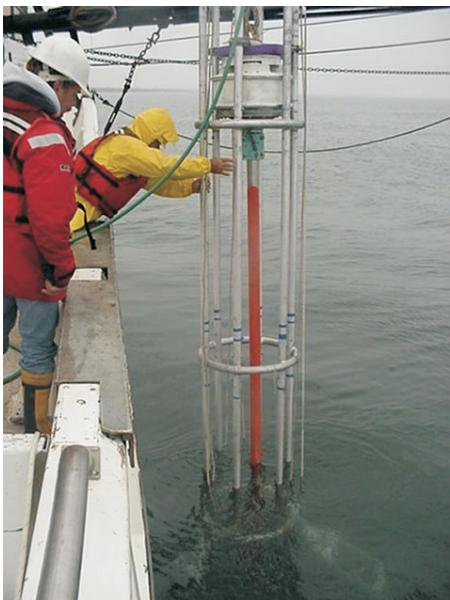
Fig. 6. Photo of vibracorer suspended at starboard side of the “Olympic”.
