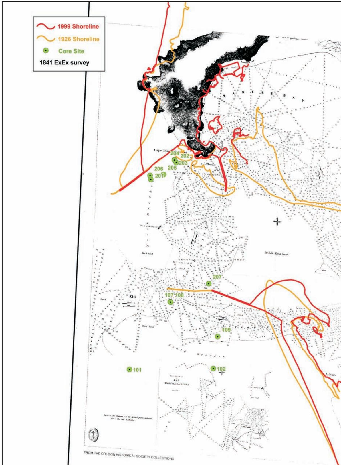
Fig. 17. Vibracore locations, jetties and 1926 and 1999 shorelines plotted on the 1841 U.S. Exploring Expedition survey by Charles Wilkes. Depths in channels are in fathoms ( $\geq 4$ ); depths on sand banks are in feet ( $\leq 23$ ).
