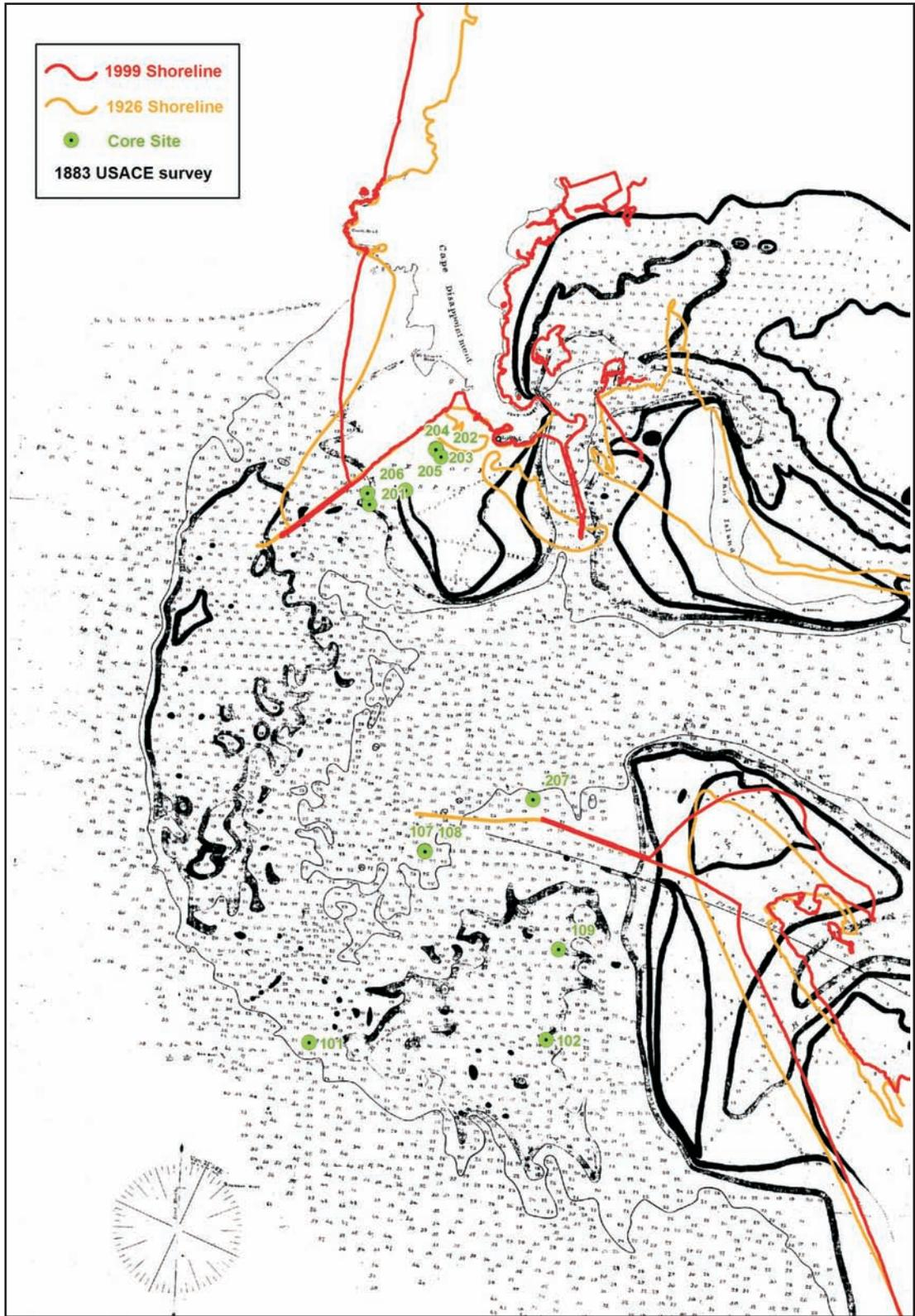
Fig. 20. Vibracore locations, jetties and 1926 and 1999 shorelines plotted on the U.S. Army Corps of Engineers survey MC-1-35 of July and August 1883. Depths are in feet below MLLW.
