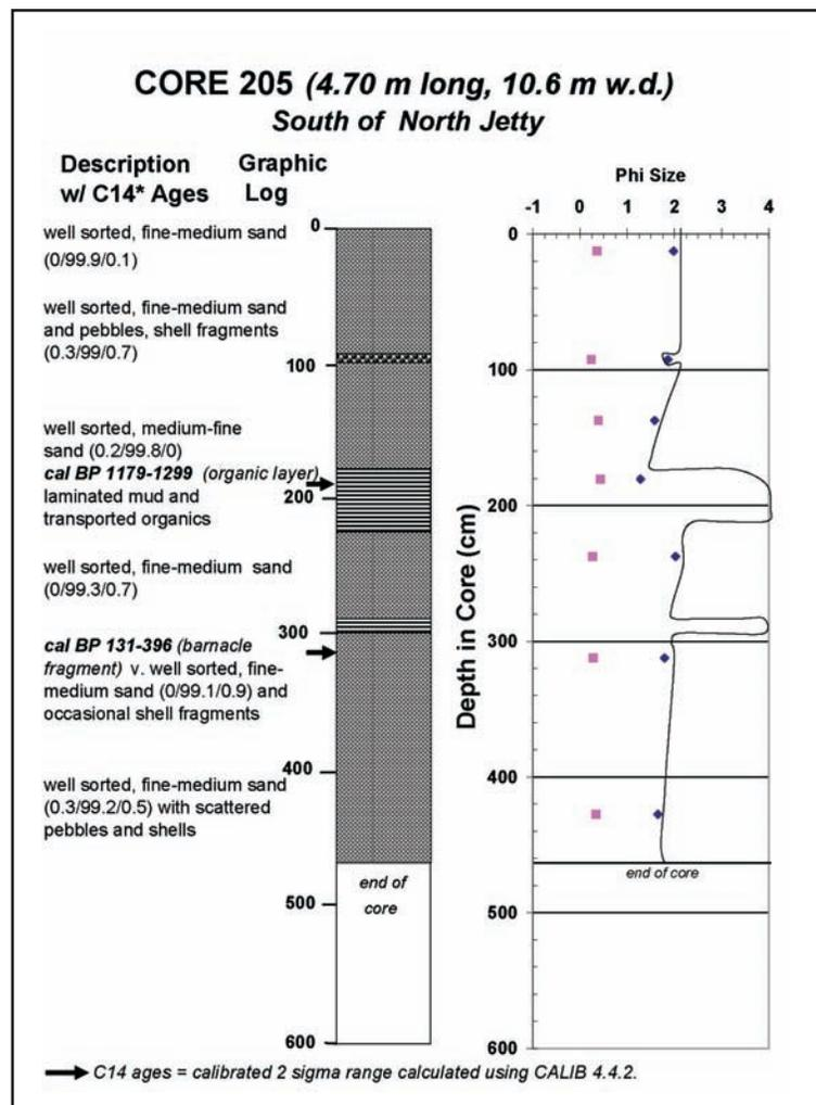
Fig. 34. Descriptive log of core MCR-205.
