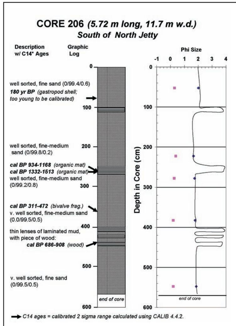
Fig. 35. Descriptive log of core MCR-206.
