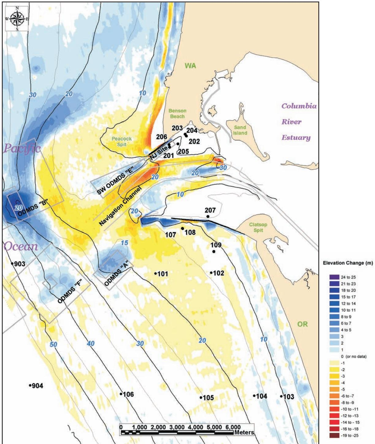
Fig. 25. Locations of vibracores collected in previous study in 2002 by the authors and this project shown with historical bathymetric change from Buijsman et al. (2003) during the period 1958 to 2000. Bathymetric contours in meters NAVD88 derived from data from 1998-2003.
