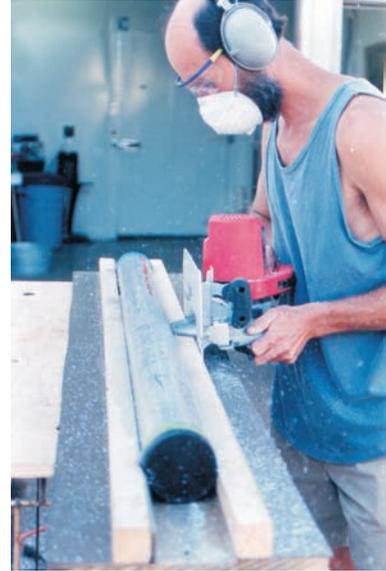
*Fig. 13. Photo of cutting core sections length-wise. Once the core barrel was cut on opposite sides, a wire was pulled through the sediment to split the core in half;*
