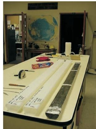
*Fig. 15. Photo of core half sealed and labeled for archiving in "D-tube".*
