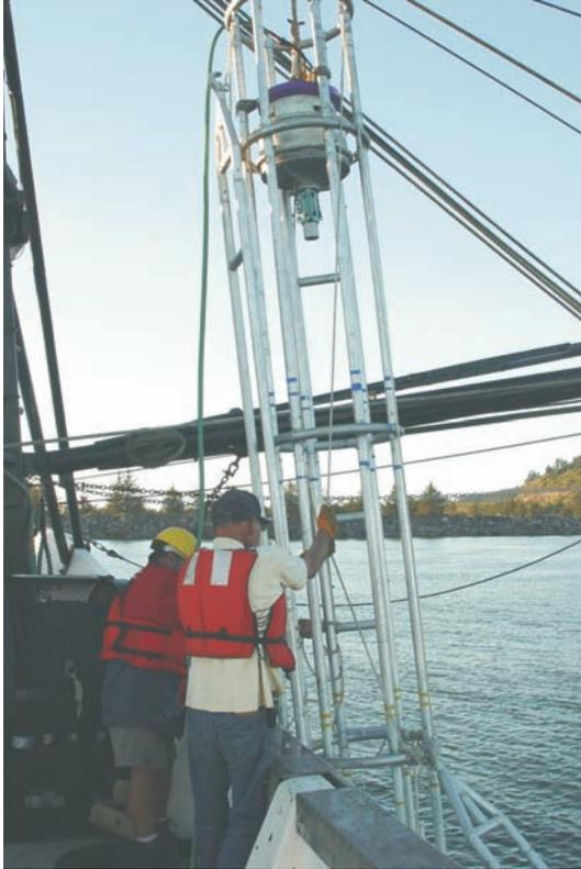
*Fig. 11. Photo of vibracorer at site C with core barrel broken off at the collar, located below the vibracorer head (photo by R. Gammisch).*
