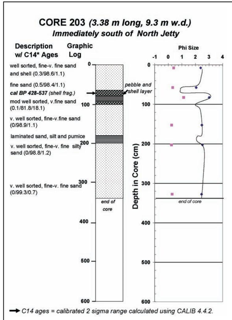
Fig. 32. Descriptive log of core MCR-203.
