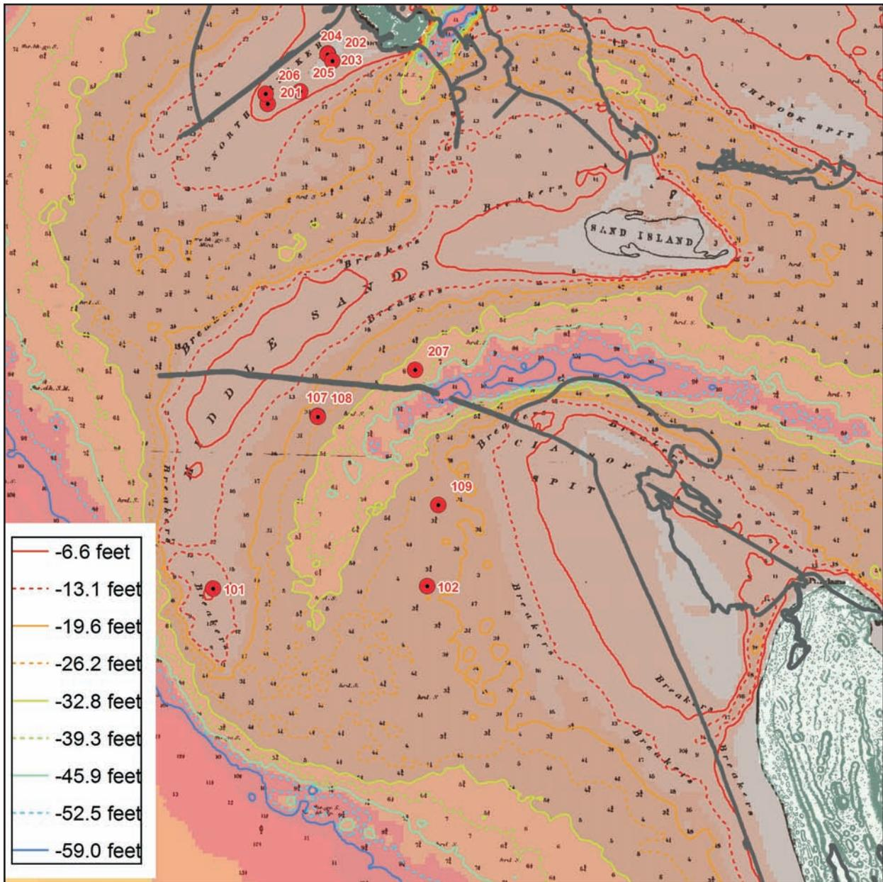
Fig. 42. Vibracore locations and 1957 jetties and shoreline plotted on 1868 bathymetry where the deepest part of the south channel passes just to the east of the “knuckle” on the south jetty. The gap in the jetty in 1957 is co-located with the deepest part of the south channel in 1868.
