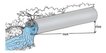
2. Once A, R and S are calculated, the values can be placed into the equation to determine discharge:
