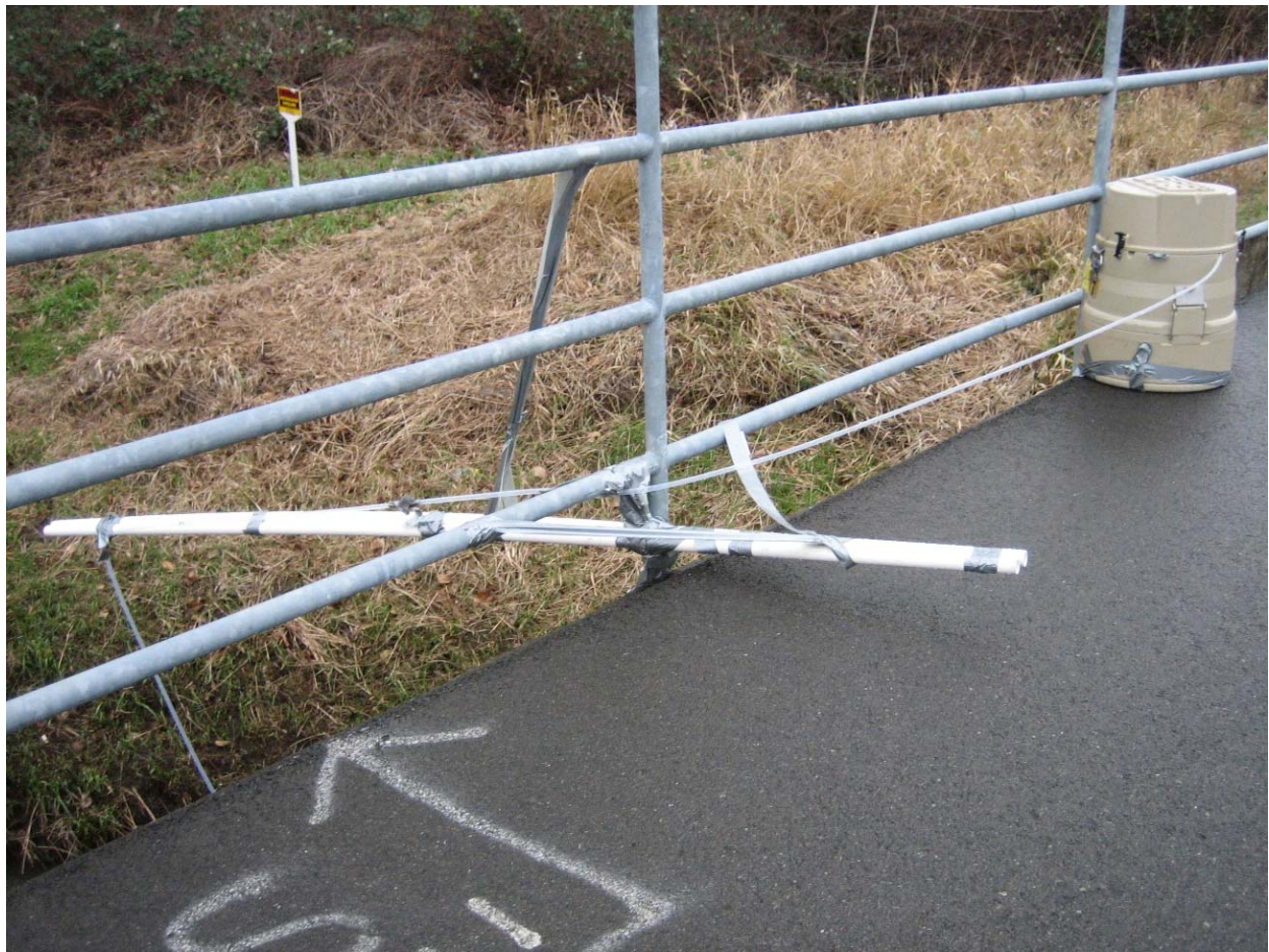
Figure 2. Setup of the portable sampler on the Interurban Trail pedestrian bridge.
