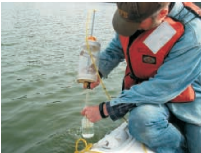
Dave Hallock uses a "Kemmerer" sampler at Lake Ballinger to collect water from a specific depth.
