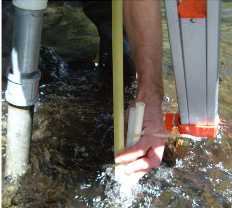
Figure A-4. Using a stilling tube to measure the operating head.
