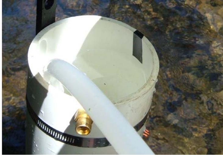
Figure A-3. Setting a constant head mark on the interior wall of the CHIT chamber.
