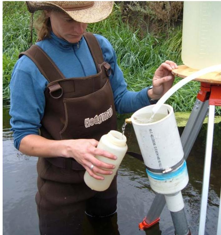
Figure A-2. Capturing the overflow ( $Q_{out}$ ) in a calibrated container during a CHIT.
