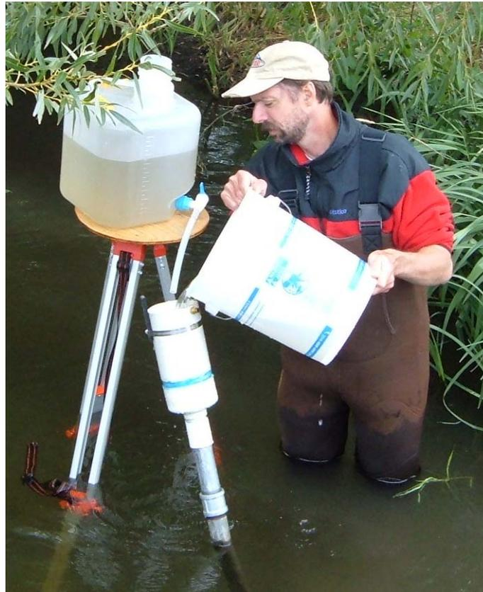
Figure A-1. Priming the piezometer and constant head chamber with clean stream water.
