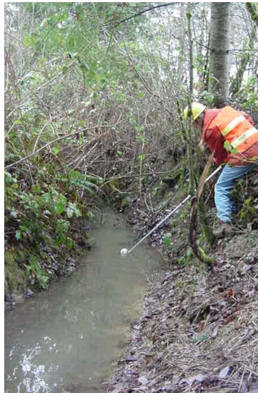
Sampling in a ditch with a collection bottle attached to a pole
