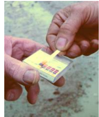
A pH strip matched to the color chart provided in the pH kit.
