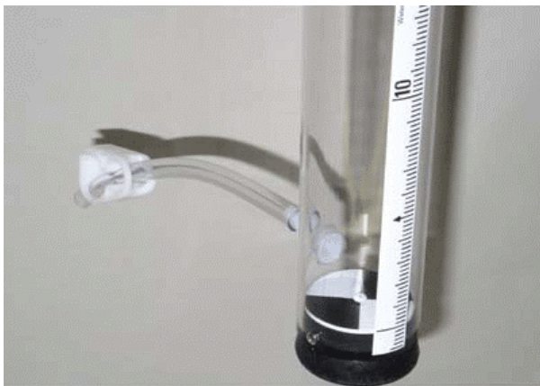
The secchi disk is the black and white disk located at the bottom of the transparency tube. Photo courtesy of: http://www.wildco.com/ow_prdct_mdl.asp?prdct_mdl_cd=58T
