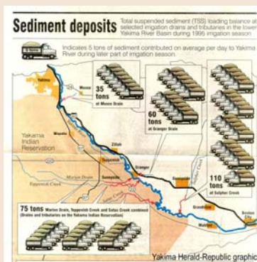
From 1995 to 2003: Irrigation improvements reduced top soil losses from 280 tons to 65 tons.
