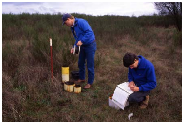
Chuck Lehotsky (left) and Kirk Sinclair measuring the groundwater level in a monitoring well near Scatter Creek in southern Thurston County.
