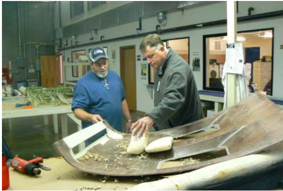
Bob Stillwell of International Aero Inc. shows Toxics Reduction staff member Tom Boucher a non-chemical paint stripping process they use.
