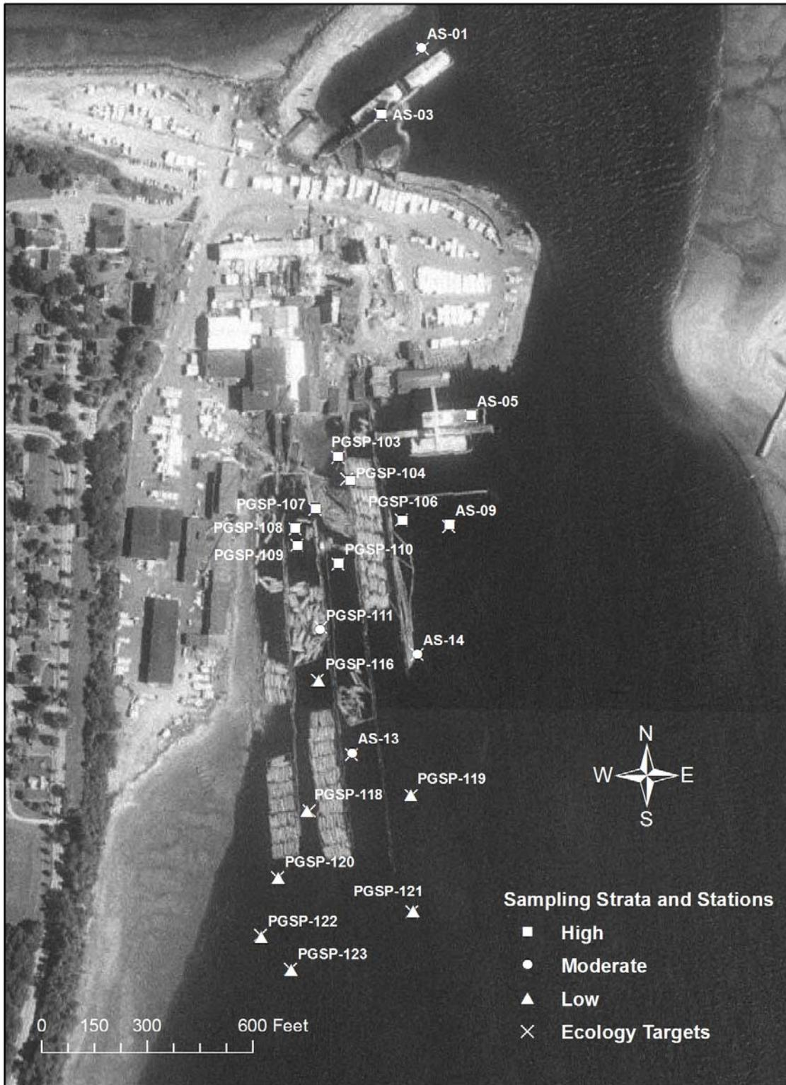
Figure 5. Aerial view of the Port Gamble Bay study site showing target and actual sediment quality sampling locations, with preliminary sampling strata indicated.
