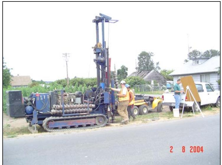
Track-mounted hollow stem auger drill rig in operation
