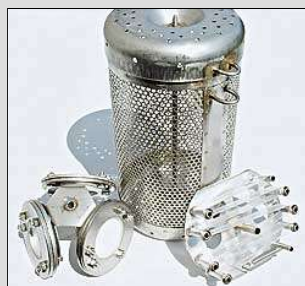
Figure 2. Left: Three POCIS on a deployment carrier. Right: SPMD on a spider carrier. Center: Protective deployment canister. (Photo courtesy of EST, www.est-lab.com ).
