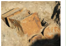
Above- Metal boxes and barrels break down and leak over time.
