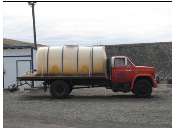
Brine application tanker truck
