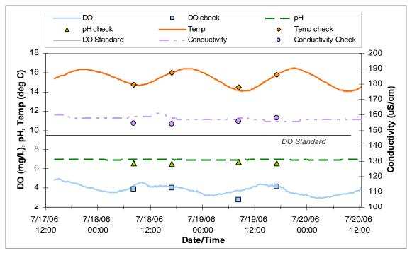
Figure C-10. Continuous 15-minute multi-parameter YSI® data for 08EVAN01.7.
