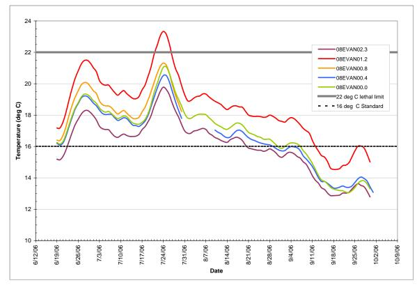
Figure B-8. Lower Evans Creek 7-DADMax of water temperature.
