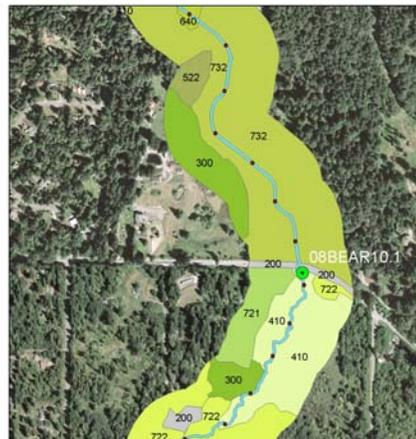
Figure 7. Steps carried out for digitizing stream channel and riparian vegetation using aerial imagery and LiDAR tree height data in GIS.
