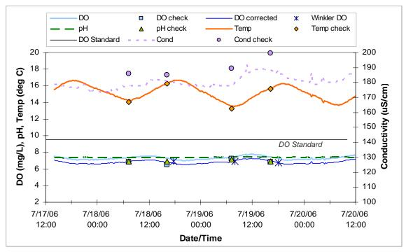
Figure C-9. Continuous 15-minute multi-parameter YSI® data for 08EVAN04.3.
