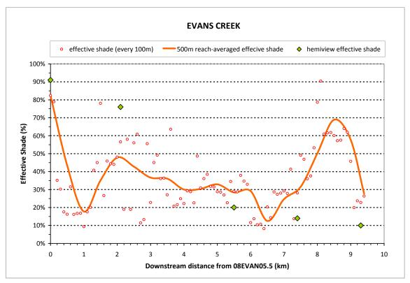
Figure 9. Current longitudinal effective shade profile for Evans Creek.
