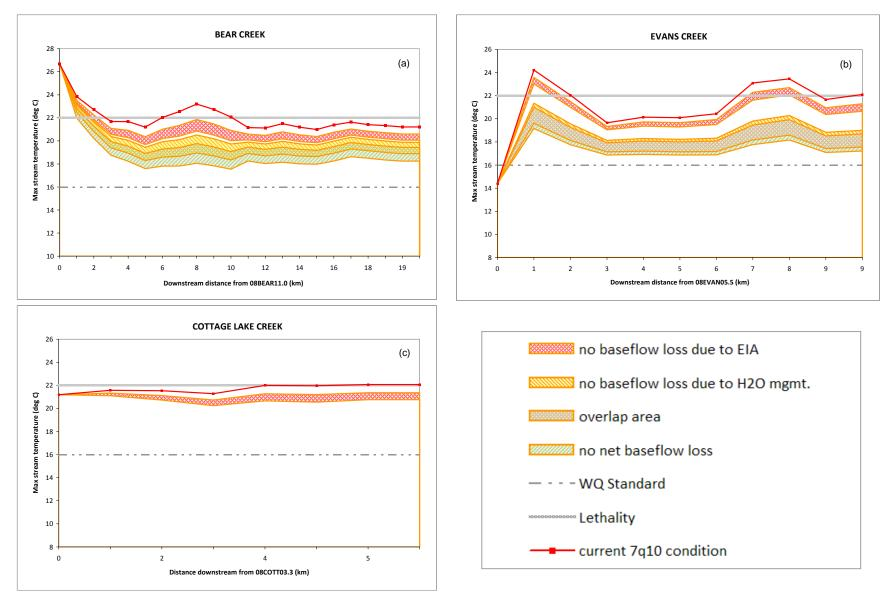
Figure 27. Range of maximum predicted stream temperatures in Bear, Evans, and Cottage Lake Creeks if there were no baseflow losses due to EIA and water management under critical conditions (range represents response to reported and conservative estimates).
