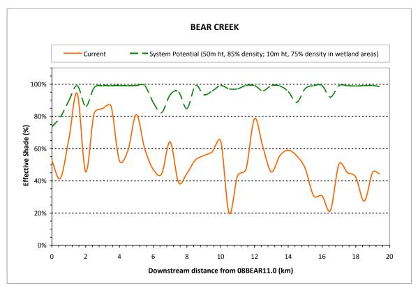
Figure 11. Current and system potential effective shade profile for Bear Creek.
