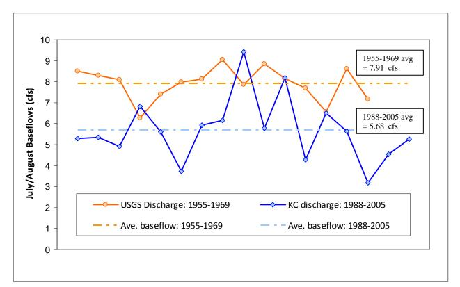
Figure 24. Comparison of 7-day average historical and current July and August baseflows near the mouth of Evans Creek based on historical USGS gage data (station #12124000) and current King County gage data (station 18a).
