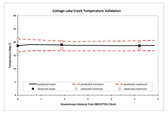
Figure 23. Comparison of predicted and observed temperatures for Cottage Lake Creek on July 21-27, 2006.
