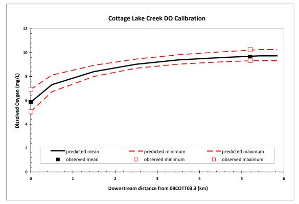
Figure 20. Comparison of predicted and observed DO for Cottage Lake Creek on July 18-19, 2006.
