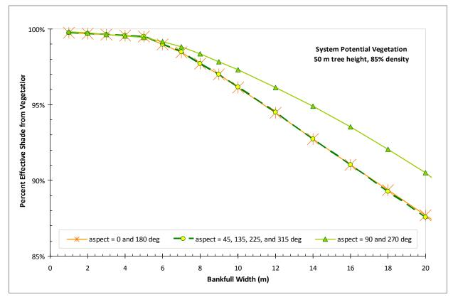
Figure 31. Load allocations for effective shade for various bankfull width and aspect of perennial streams and tributaries to mainstem Bear, Evans, and Cottage Lake Creeks.
