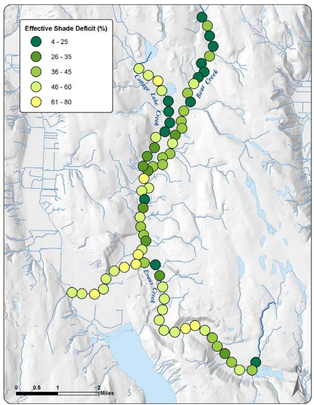
Figure 32. Effective shade deficits in the Bear-Evans watershed based on the difference between current and system potential mature riparian vegetation.
