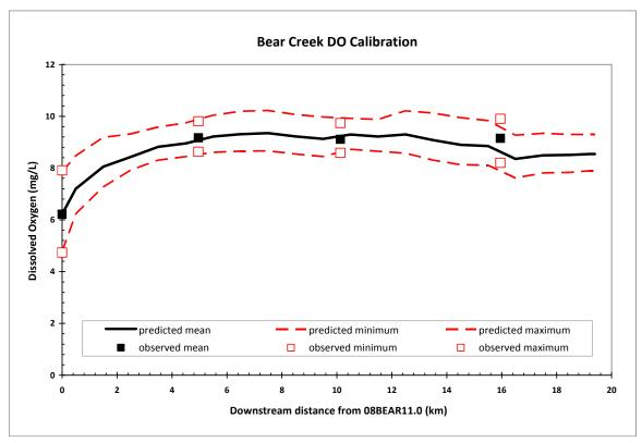
Figure 18. Comparison of predicted and observed DO for Bear Creek on July 18-19, 2006.
