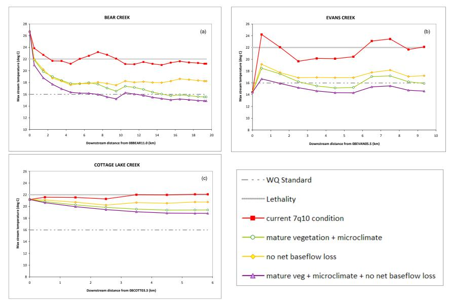
Figure 28. Maximum predicted stream temperatures in Bear, Evans, and Cottage Lake Creeks with implementation of mature vegetation and microclimate improvements combined with no net baseflow losses (conservative estimate).
