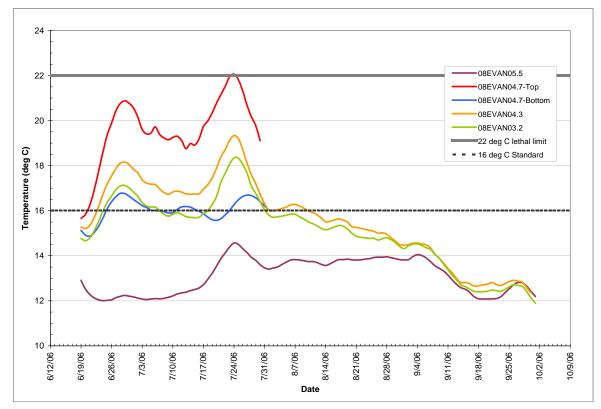
Figure B-7. Upper Evans Creek 7-DADMax of water temperature.
