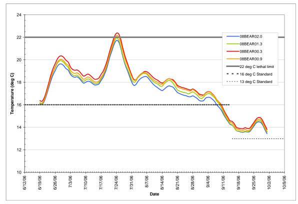
Figure B-3. Lower Bear Creek 7-DADMax of water temperature.
