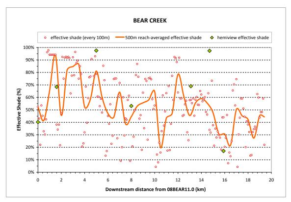
Figure 8. Current longitudinal effective shade profile for Bear Creek.
