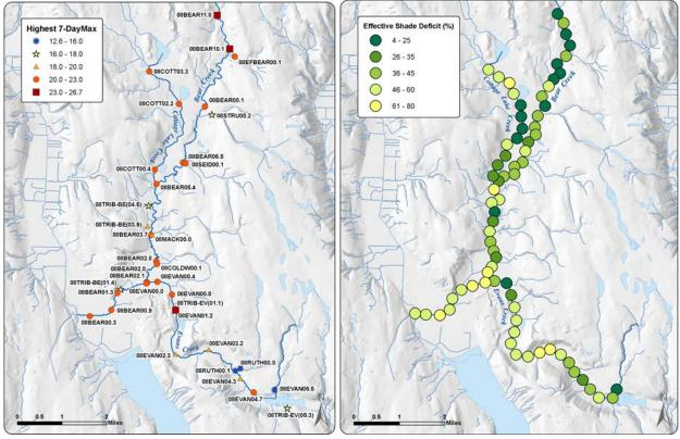
Figure ES-3. Highest 7-DADMax temperatures recorded. Figure ES-4. Effective shade deficits and shade load allocations.
