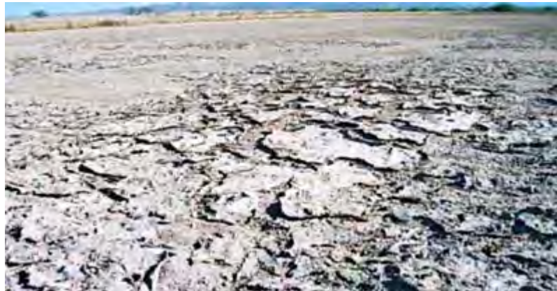
Desiccation cracks formed on basin bottom from drying the clogging layer.
