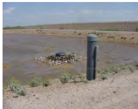
Basin stilling well with pressure transducer mounted inside to measure water levels in the basin (Basin 2B)
