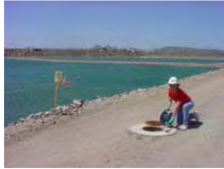
Water Level Monitoring Being Conducted at Recharge Basins
