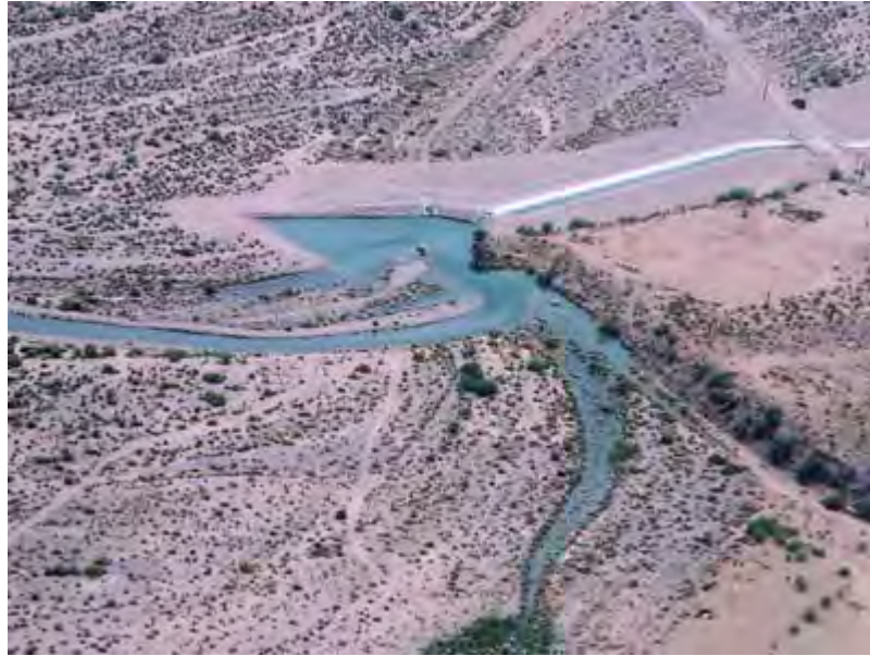
Water Captured from River at Headworks Structure for Delivery to Recharge Basins
