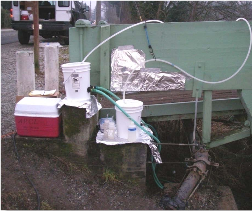
Figure B-6. Sieving station at end of sampling site footbridge.
