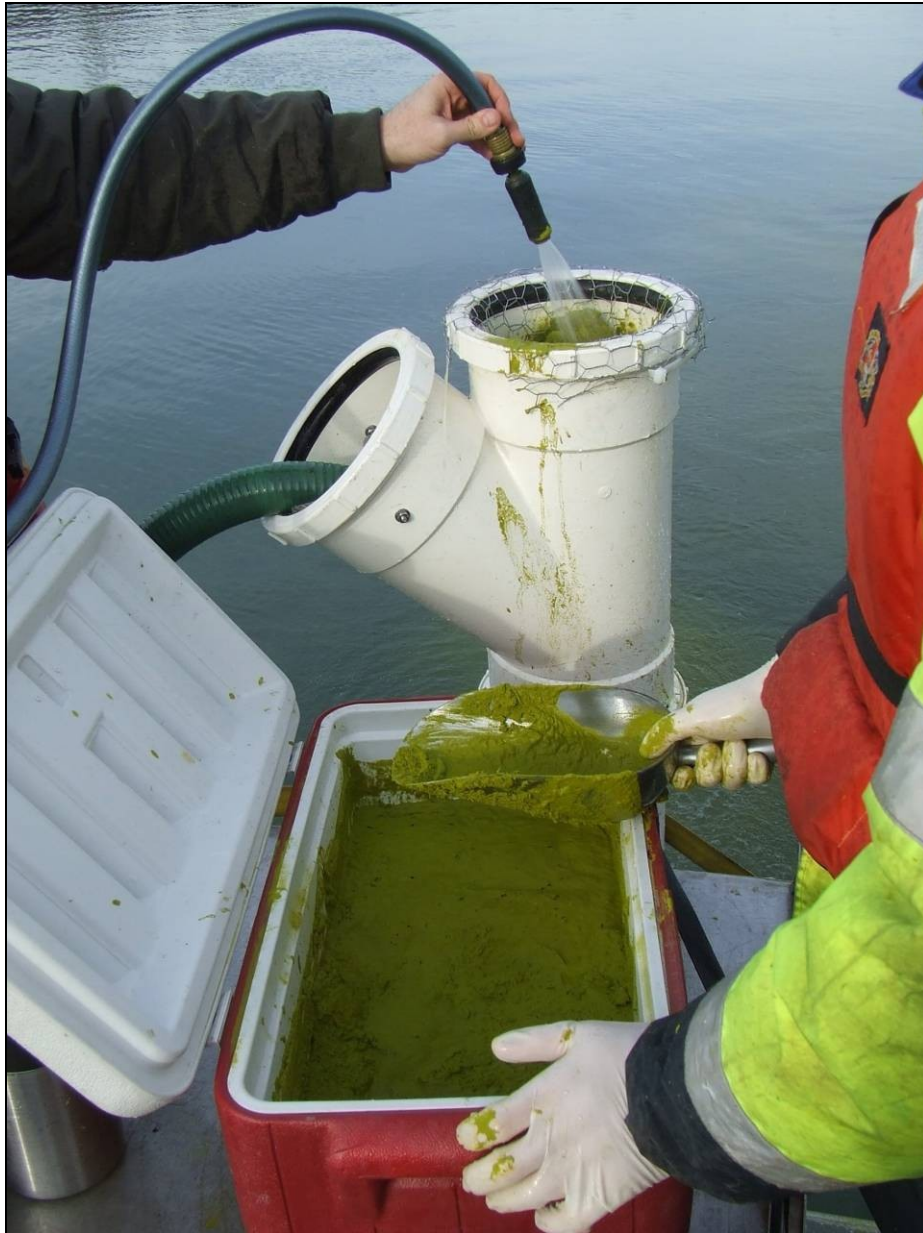
Figure 8 Photograph showing the method of introduction of tracer. The tracer is scooped from the cooler boxes and flushed down the tube using a low-flow hose; tracer enters the water sub-surface.
