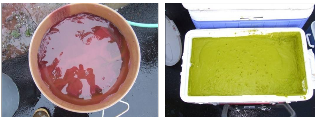
Figure 7 Plan view of both the sand (red) and silt (green) tracers in a cool-boxes following pre-wetting and prior to injection.
