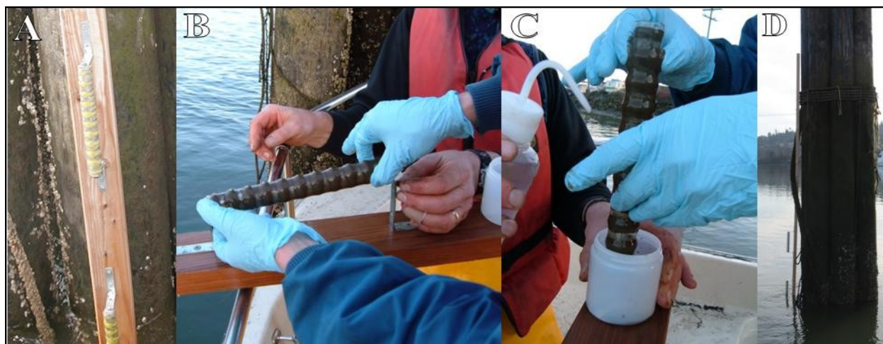
Figure 11 Magnet sampling images: A) Bar magnets mounted to a piling with visible yellow silt tracer, B) Removing the plastic sheath from magnet, C) Rinsing sheath into a plastic jar, D) Magnets mounted on piling (images courtesy of Ecology).
