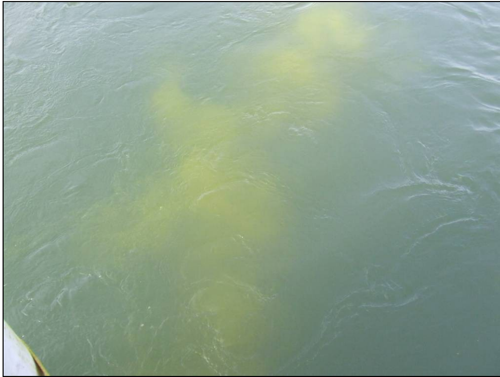
Figure 9 Photograph of the sub-surface plume of silt tracer formed during injection of the tracer material.
