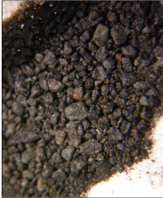
Figure 4 Microphotograph of naturally occurring magnetic material from bedded sediments in the LDW. The largest grain in the centre of the image is ca. 120 \mu\text{m} in diameter.
