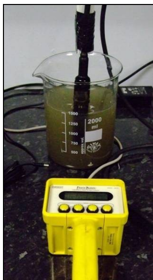
Figure 9. Silts settling velocity set-up. Figure 10. Dataron screen.
