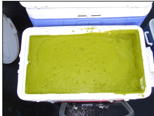
Figure 10 Plan view of the silt tracer in a cool-box prior to injection.
