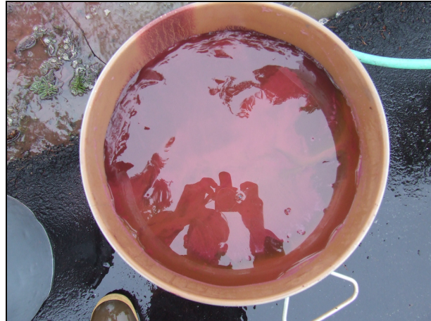
Figure 6 Plan view of the sand tracer in a drum prior to injection. The tracer was observed macroscopically to behave like mineral sand (naturally slightly compact, moisture redistribution upon disturbance, temporary clumping when troweled into the injection funnel).
