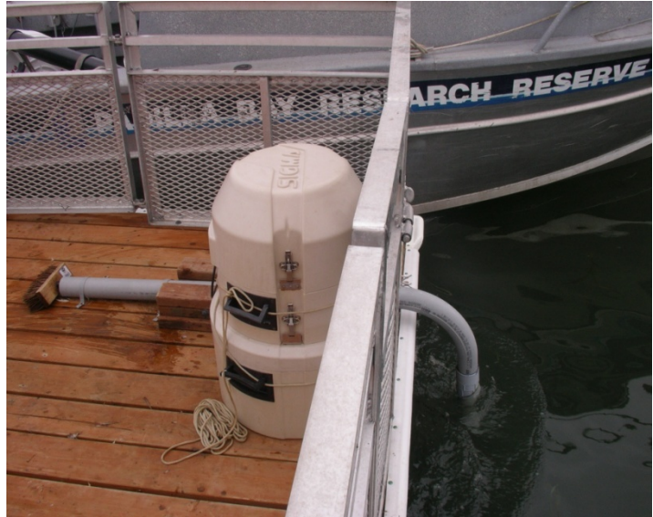
An automatic sampler collects 24 water samples for nutrient analyses over one 26-hour tidal cycle each month.
