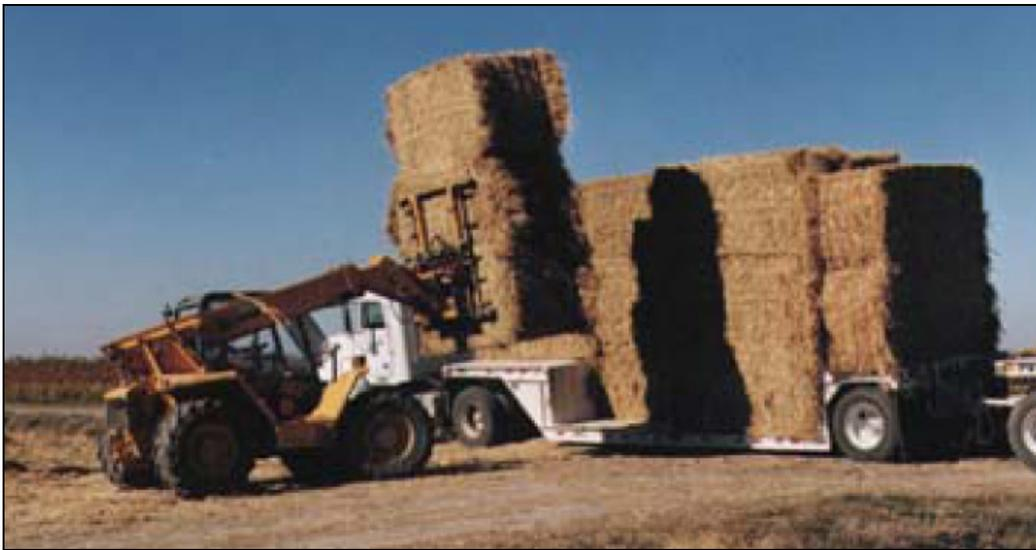
Figure 112: Loading Drop-Bed Trailer Truck (Large Bales: 1.2 × 1.2 × 2.4 m)
