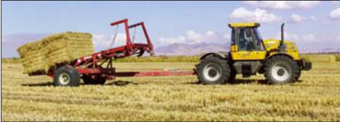
Figure 111: Road-Siding Process (Large Bales: 1.2 × 1.2 × 2.4 m)
