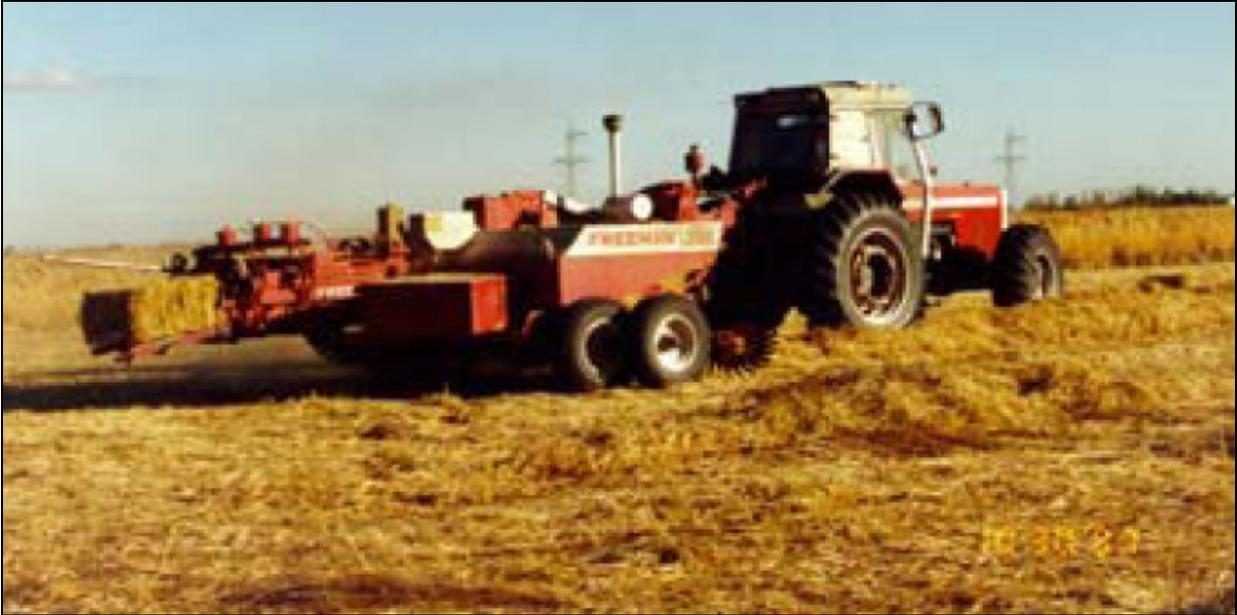
Figure 109: Baling Process (Small Bales:  $0.4 \times 0.6 \times 1.2$  m)
