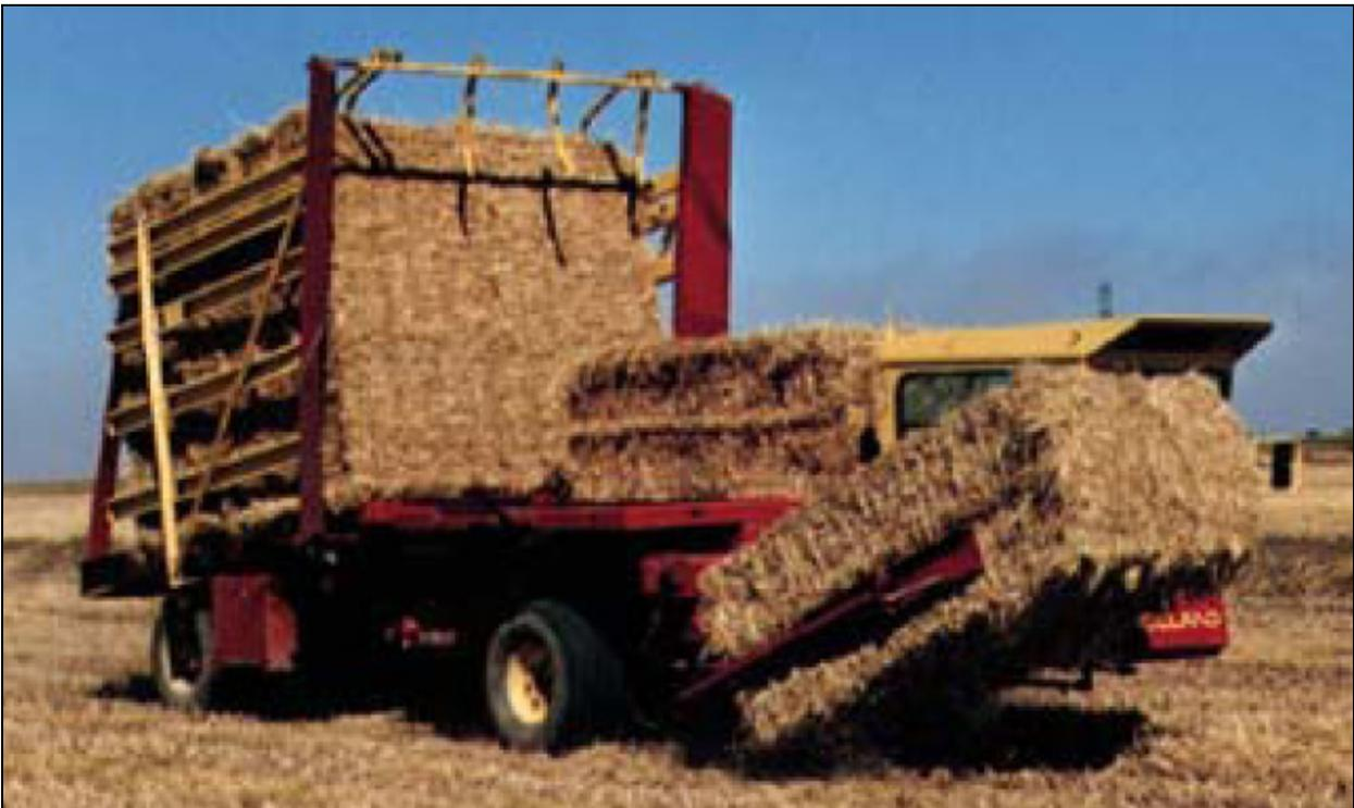
Figure 110: Road-Siding Process (Large Bales:  $1.2 \times 1.2 \times 2.4$  m)
