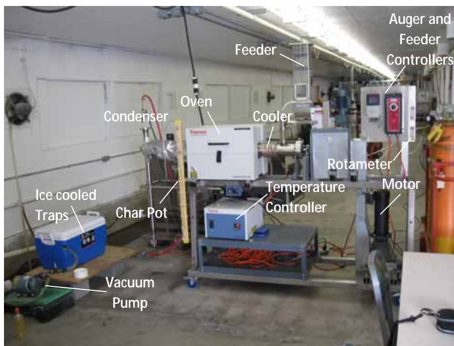
Figure 3.8.- Picture of the new Auger Pyrolysis reactor operational at WSU.
