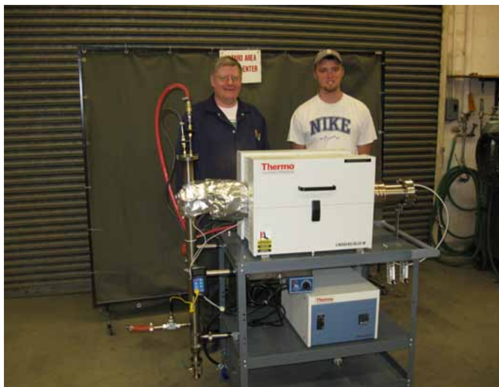
Figure 3.6.- Picture of the Batch Pyrolysis Reactor built at WSU (Mr. Wayne Dewitt and Mr. Brandon Kruger).
