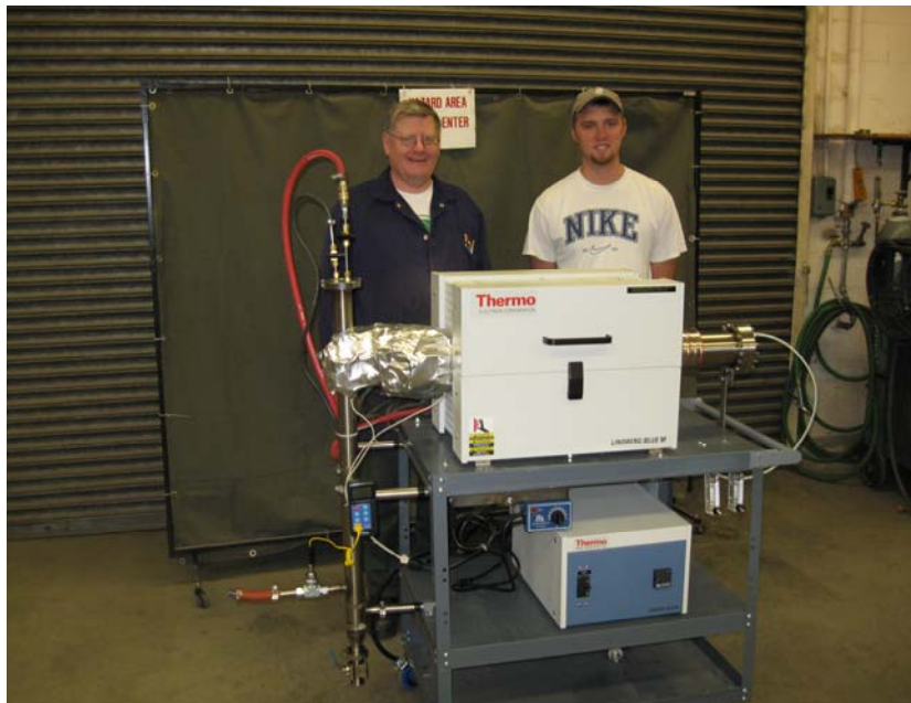
Figure 2.2. Photo of the Batch Pyrolysis Reactor built at WSU.
