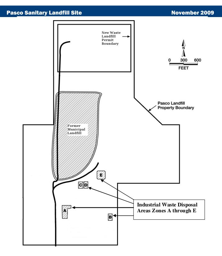
Figure 4 Landfill Waste Sections and Zones
