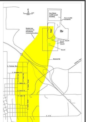
Figure 1 Groundwater Contamination Plume 4<sup>th</sup> Quarter 1996
