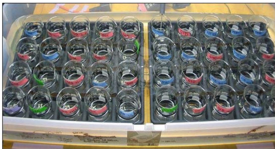
Figure 4. Example of one WET test replicate (bottom photo). Two trays with test chamber positions numbered 1-40 (top photo) were used to accommodate test chambers in a static water bath (bottom photo). Colors illustrate different solution types (purple = fluoranthene reference control; green = negative dilution water control; blue = positive reference control; red = groundwater).
