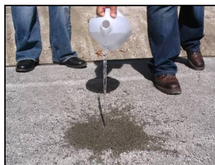
Demonstrating the infiltration of the permeable concrete.
