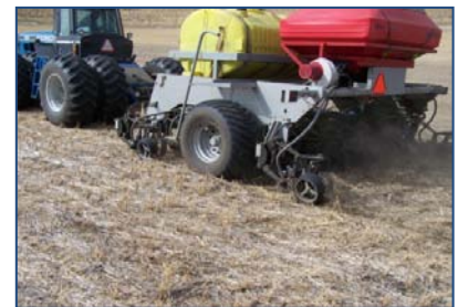
Direct seed drill at work. Note the relatively undisturbed soil.
