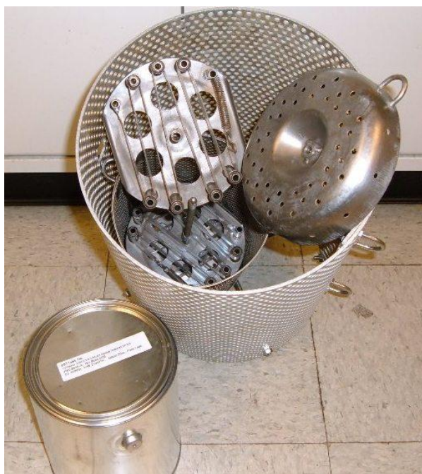
Figure 3. SPMDs Inside a 5-membrane Canister and Inserted in a Shade Device Cylinder.
