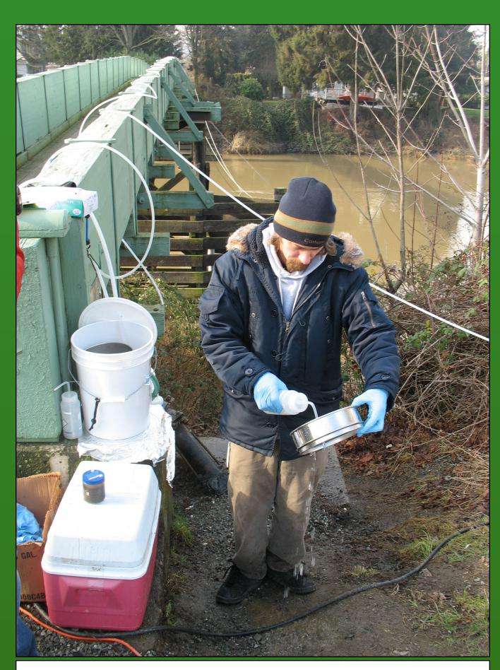
Figure 7. Collecting sediment from sieves. Suspended sediments collected on sieves were rinsed with site water into pre-cleaned glass jars.
