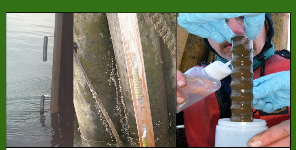
Figure 11. Left to right: Magnet samplers before being deployed, with silt tracers, and tracer recovery.
