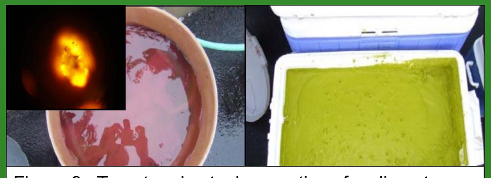
Figure 9. Target and actual properties of sediment tracers, with images of indivdual particles and pre-wet batches ready for release.
