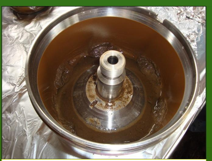
Figure 5. View inside centrifuge bowl after removing overlying water.
