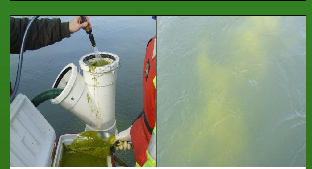
Figure 10. Release of yellow-green sediment tracers, representing native silts, to form subsurface plume.
