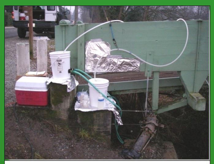
Figure 6. Flow-through sieving station. River water was pumped through 1-2 stainless steel sieves for timed intervals until centrifuge sampling ended.
