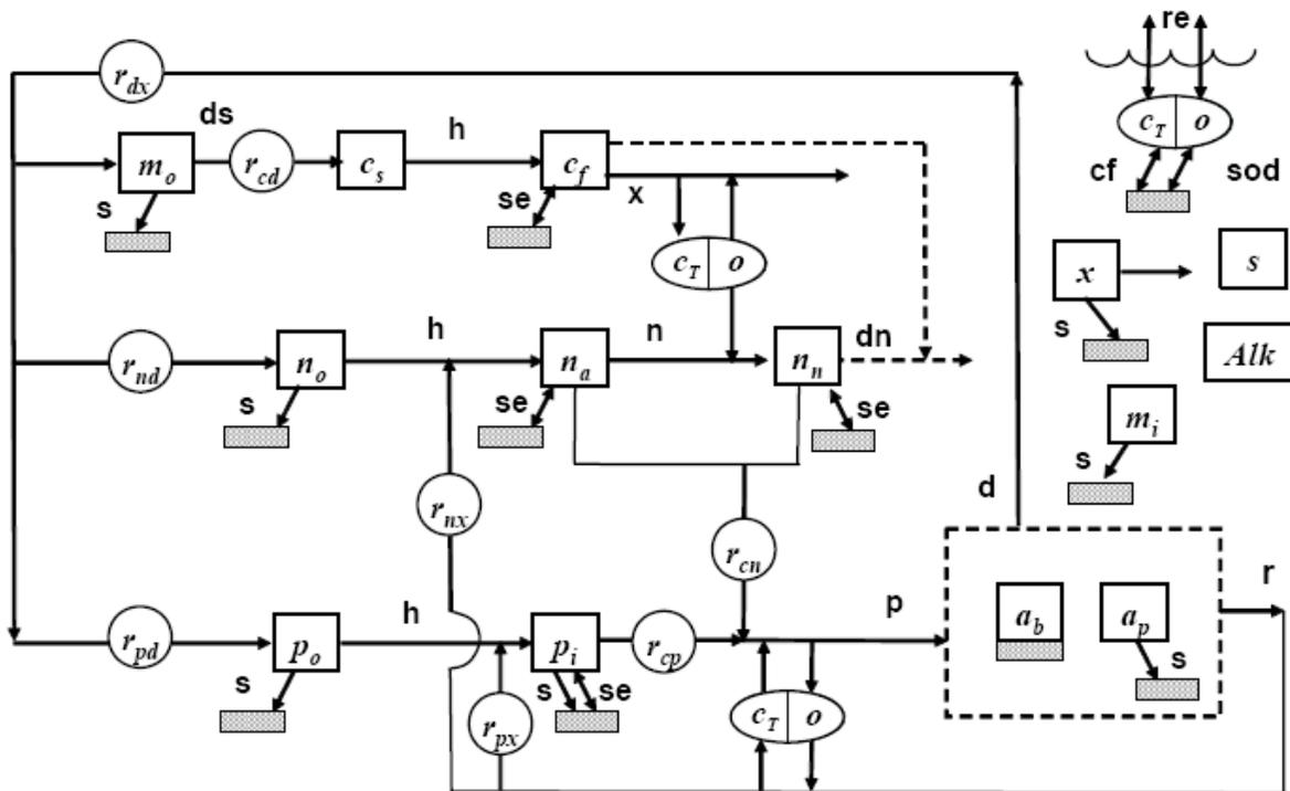
**Figure 10. Model kinetics and mass transfer processes in QUAL2Kw.**
