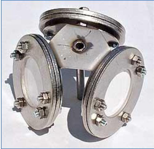
Figure 5. Three Standard POCIS Membranes on a Deployment Carrier.
