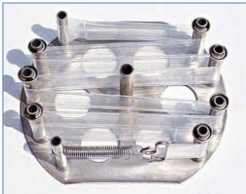
Figure 4. Standard SPMD Membrane Mounted on a Spider Carrier.
