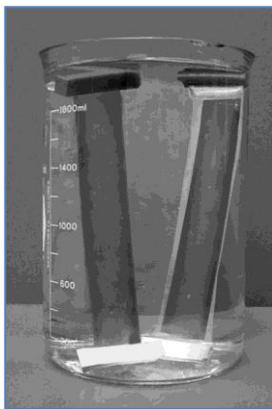
Figure 9. Sheathed Bare SLMD Membranes.
