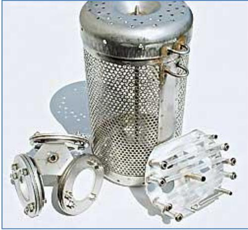
Figure 8. Large Canister Which Can Fit Both POCIS (left) and SPMD (right) Membranes Together.
