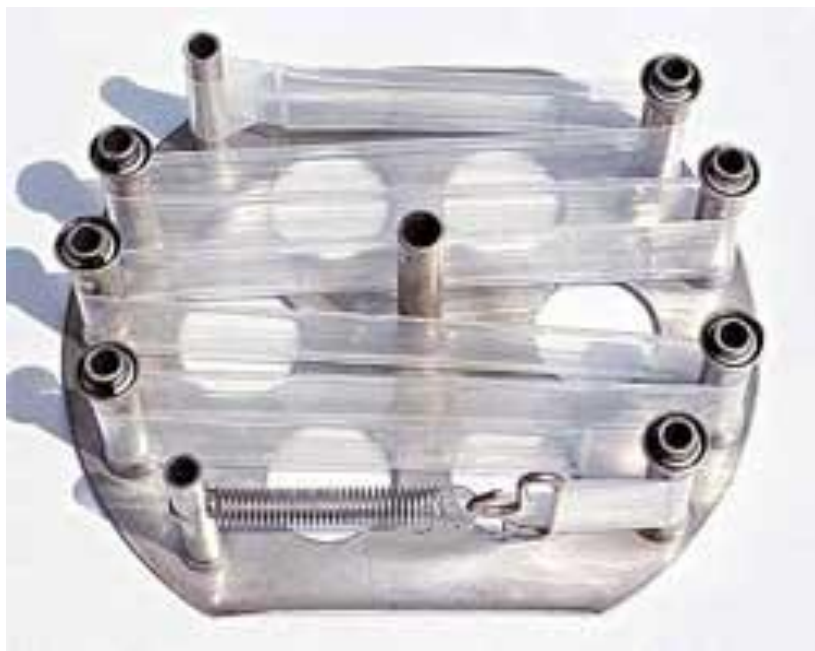
Figure 5. Standard SPMD Membrane Mounted on a Spider Carrier.
