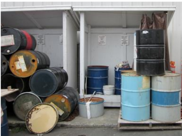
Unsafe storage of dangerous waste
