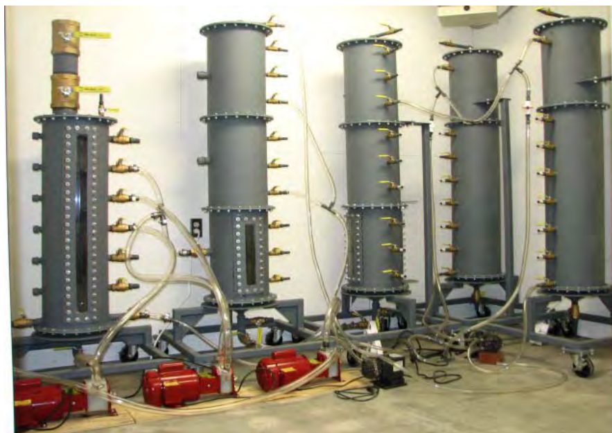
Moderate High Solids Anaerobic Digester floor scale laboratory digester under testing at WSU Biological Systems Engineering Department.
