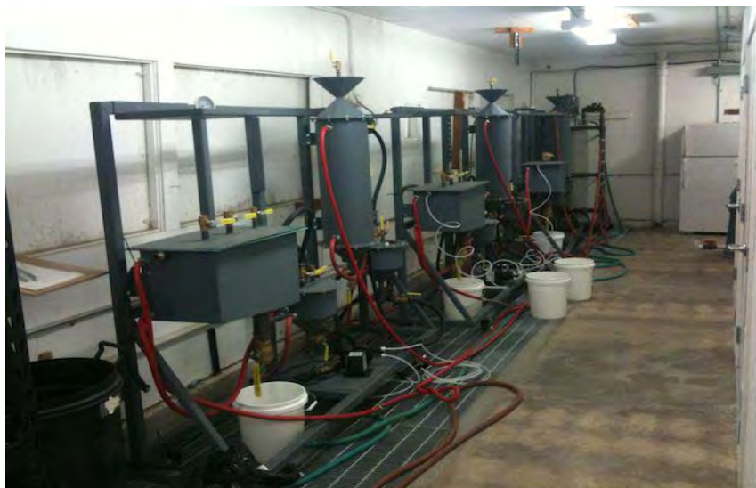
High Solids Anaerobic Digester floor scale laboratory digester under testing at WSU Biological Systems Engineering Department.
