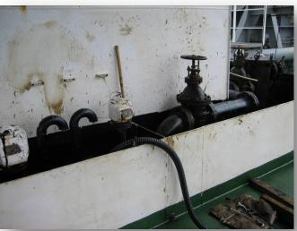
Figure 3 - The No. 4 starboard main deck fuel oil tank valve.
