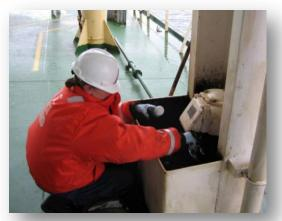
Figure 5 - A U.S. Coast Guard (USCG) officer takes a sample from the No. 4 starboard fuel oil vent containment box.
